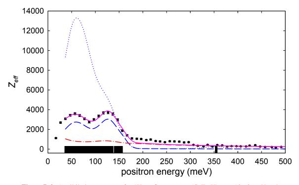
**Figure B.2**: Annihilation spectrum for 1H-perfluorooctane (C<sub>8</sub>F<sub>17</sub>H):  $\varepsilon_b = 19 \pm 3$  meV and  $\eta = 0.70$ .
