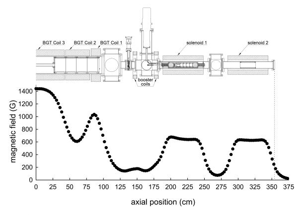
**Figure 7.5**: Measured magnetic field of CBT-based beamline. (Top) schematic diagram of the beamline from the second stage of the BGT to the RPA region and (bottom) measured on-axis magnetic field over the same region under typical conditions. Vertical dashed line indicates relative position of end of beamline.
