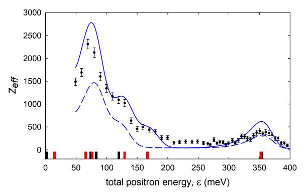
**Figure 4.2**: Annihilation spectrum for 1,2-trans-dichloroethylene ( $C_2H_2Cl_2$ ); (•) measured data, (––) GL model from Eq. (A.8) with  $\varepsilon_b = 29$  meV using infrared-active modes only and (—) GL model using all modes. Vertical bar positions represent vibrational mode energies downshifted by the binding energy, and heights represent mode degeneracies. Black and red indicate infrared-active and inactive modes, respectively.
