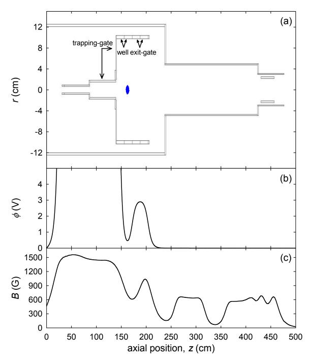
**Figure 5.1**: BGT-based beamline simulation initial conditions. (a) electrode geometry with ( $\bullet$ ) positron initial axial and radial positions, (b) initial on-axis potential and (c) axial magnetic field. For this example, the trapping-gate, well and exit-gate electrodes are set to 30, 0 and 3 V respectively.
