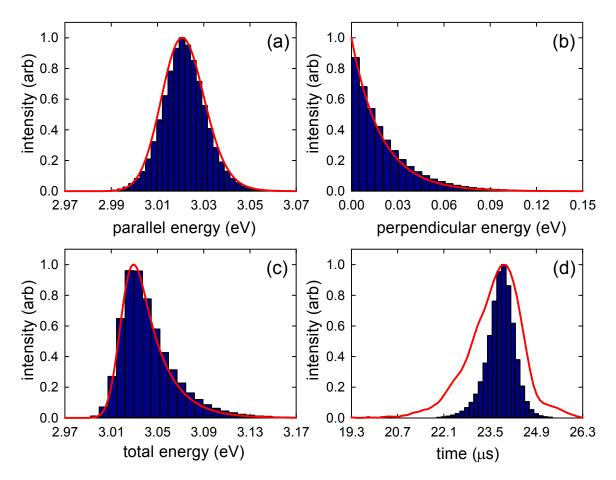
**Figure 5.5**: BGT distributions obtained from experiment and simulation for the conditions described by Figs. 5.1-5.4. (a) parallel energy, (b) perpendicular energy, (c) total energy, and (d) time. Blue bars represent simulation results, and red lines show experimental measurements. See text for details.
