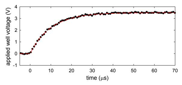
**Figure 2.6**: Typical BGT ejection ramp function. (•) applied voltage as measured on an oscilloscope, and (– –) Eq. (2.2) with  $V_s = 3.5$  V,  $V_0 = 0$  V and  $\tau_r = 10 \ \mu$ s.
