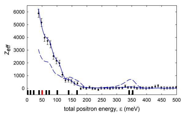
**Figure 4.4**: Annihilation spectrum of 1,1-dichloroethylene (C<sub>2</sub>H<sub>2</sub>Cl<sub>2</sub>); (•) measured data with the fitted MRA component subtracted for clarity, (––) GL model from Eq. (A.8) with  $\varepsilon_b = 31$  meV, (––) scaled GL model from Eq. (A.15). Vertical bar positions represent vibrational mode energies downshifted by the binding energy and heights represent mode degeneracies, where black and red indicate infrared-active and inactive modes, respectively.
