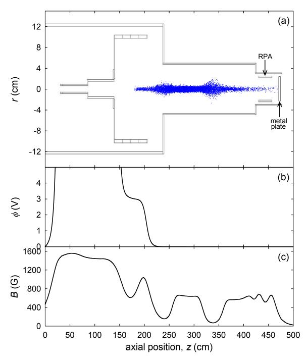
**Figure 5.4**: BGT-based beamline simulation beam transport. (a) electrode geometry with (•) positron axial and radial positions, (b) on-axis potential, and (c) on-axis magnetic field at  $t = 22 \ \mu$ s, under the conditions described in Fig. 5.1 and 5.2.
