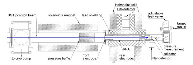
**Figure 2.8**: Schematic diagram of the annihilation region. A solenoidal magnet and a set of Helmholtz coils provide a magnetic field which varies between 500 and 700 G, while the front and rear electrodes, the RPA, collector and NaI gamma-ray detector are used to diagnose the BGT beam. The leak valve, pressure baffle, lead shielding, and CsI gamma-ray detector are used for positron annihilation studies.
