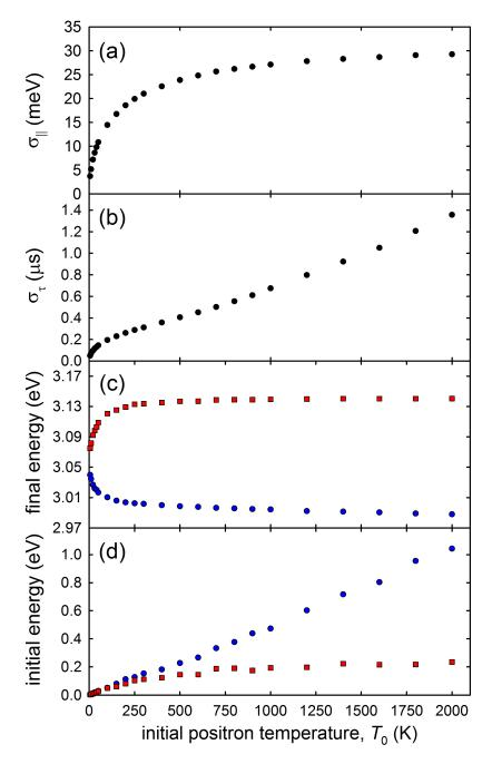
**Figure 5.11**: Effect of positron temperature on simulated beam. Standard deviations of the (a) parallel energy and (b) temporal distributions obtained from the simulation of beams generated using various initial particle temperatures. Also shown is the (c) final and (d) initial parallel energies of the particles which are ejected with the (•) lowest and (•) highest final parallel energies in the beam. All other parameters as in Fig. 5.8.
