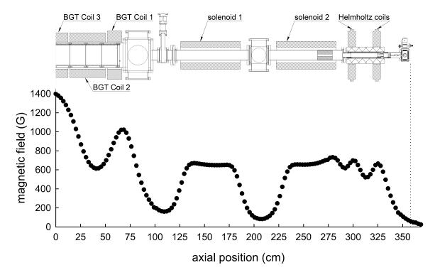
**Figure 2.7**: Measured magnetic field of BGT-based beamline. (Top) schematic diagram of the beamline from the third-stage of the BGT to the annihilation region, and (bottom) measured on-axis magnetic field under typical conditions over this region. Vertical dashed line indicates relative position of the end of the beamline.
