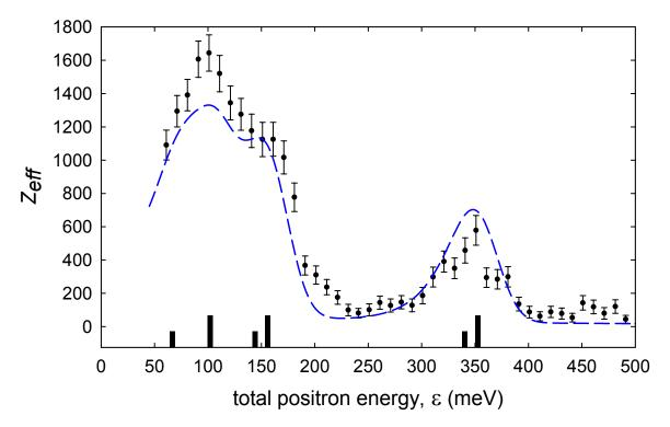
**Figure 4.1**: Annihilation spectrum for methyl chloride (CH<sub>3</sub>Cl) [33]; (•) measured data and (– –) GL model from Eq. (A.8) with  $\varepsilon_b = 24$  meV. Vertical bar positions represent vibrational mode energies downshifted by the binding energy and heights represent mode degeneracies.
