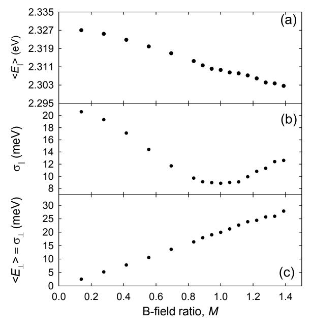
**Figure 3.6**: BGT beam measurements at various magnetic field ratios. (a) mean parallel energy, (b) standard deviation of the parallel energy distribution, and (c) mean perpendicular energy (calculated using Eq. (3.20)) at various magnetic field ratios,  $M = B_{RPA}/B_{BGT}$ . Note that, for the case of a MB perpendicular distribution,  $\overline{E}_{\perp} = \sigma_{\perp}$ .
