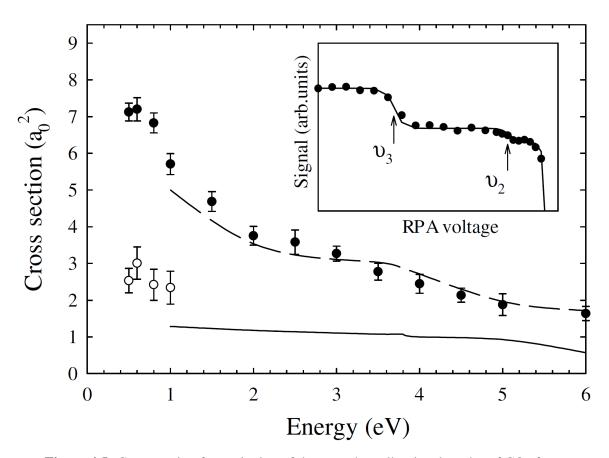
**Figure 4.5**: Cross section for excitation of the  $v_2$  and  $v_3$  vibrational modes of CO<sub>2</sub> from Ref. [16]. ( $\circ$ ) and ( $\bullet$ ) are experimental data for the  $v_2$  and  $v_3$  modes, respectively. (—) and (––) are theory from Kimura *et al.* [42] for the same two modes. Inset shows raw RPA data, showing steps due to both vibrational modes, with the solid line showing the fitted curve.
