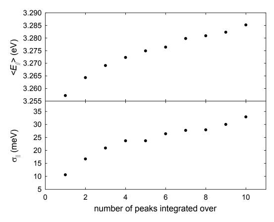
**Figure 3.8**: Effect of beam reflections on measured parallel energy distribution. (a) mean and (b) standard deviation of the parallel energy distribution as the time window of integration is increased to include multiple peaks (i.e., "secondary" beams). See text for details.
