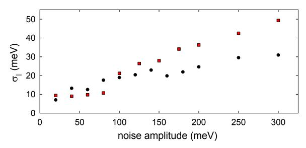
**Figure 3.9**: Effect of electronic noise on measured parallel energy distribution. Measured standard deviation of the parallel energy distribution as Gaussian noise is applied to the (●) exit-gate and (■) RPA. The horizontal axis is the peak-to-peak noise amplitude, as measured on an oscilloscope.
