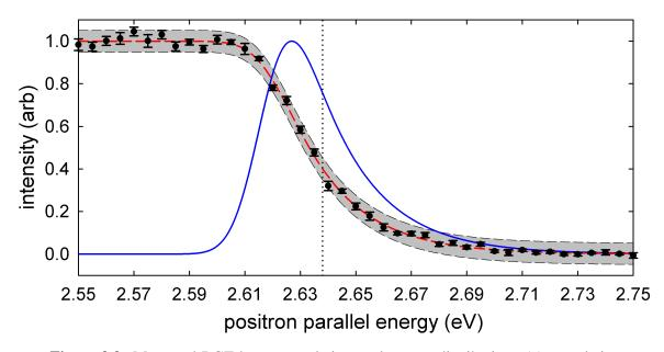
**Figure 3.3**: Measured BGT beam cumulative total energy distribution. (•) cumulative energy distribution measured at an RPA magnetic field of  $B \sim 20$  G ( $M \approx 1/30$ ), (--) EMG fit to data (Eq. (3.14). Measurements are at a sufficiently reduced field to effectively provide a measure of the total energy distribution. Shaded areas and vertical dotted lines show the 95 % confidence interval and mean parallel energy obtained from the fit.
