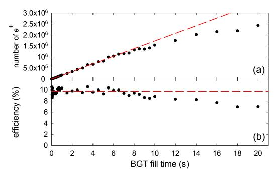
**Figure 2.5**: Typical BGT fill parameters, where (a) is the number of positrons accumulated and (b) is the trapping efficiency obtained using various BGT fill times. Red dashed lines show (a) linear fit to data and (b) mean trapping efficiency below ~ 6s.
