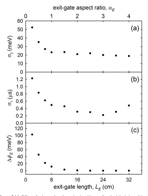
**Figure 5.14**: Effect of exit-gate length on simulated beam. Standard deviation of the (a) parallel energy and (b) time distributions obtained from the simulation of beams produced by traps with a variety of exit-gate electrode lengths. Also shown in (c) is the change in magnitude of the peak in exit-gate potential during particle ejection. All other parameters as in Fig. 5.8.
