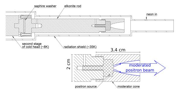
**Figure 2.2**: Schematic diagram of the source and moderator assembly. The <sup>22</sup>Na source and copper moderator cone are attached through an elkonite rod to the second-stage of a two-stage cryocooler which is maintained at 8 K. The assembly is surrounded by a radiation shield which is attached to the first-stage of the cryocooler and maintained at  $\sim 35$  K.
