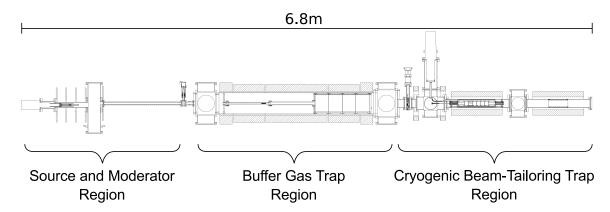
**Figure 7.1**: Schematic diagram of the CBT-based beamline. A steady-state positron beam is produced in the source and moderator region and guided into the buffer gas trap region, where it is converted into a high resolution pulsed beam. This pulsed beam is then guided into the cryogenic beam-tailoring trap region, where it is further tailored into a pulsed beam with superior characteristics.
