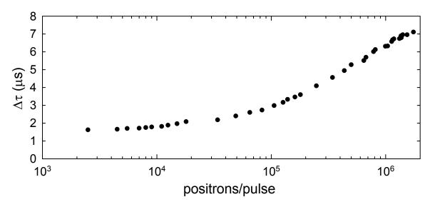
Figure 3.7: BGT temporal spread dependence on positrons number.
