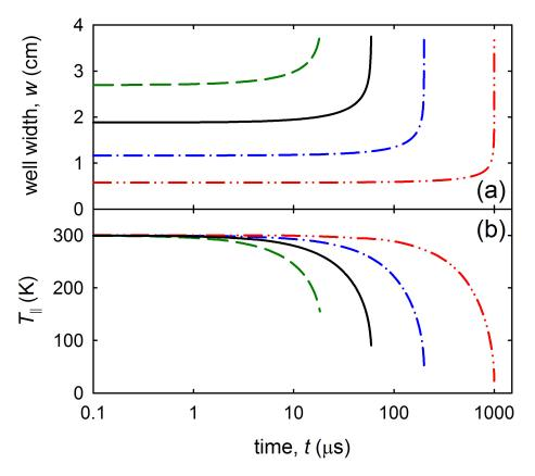
**Figure 5.13**: Effect of well depth on beam formation. (a) average potential well width as seen by the particles and (b) particle parallel temperature as a function of time obtained from the simulation using an initial well depth of (--) 1 V, (-) 3 V, (--) 10 V and  $(-\cdots -)$  50 V.
