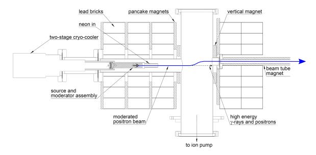
**Figure 2.3**: Schematic diagram of the source and moderator region. The source is vertically offset from the beam tube magnet to break line-of-sight with the downstream beamline. A series of pancake magnets generate a  $\sim 150$  G magnetic field for radial confinement of the moderated positrons, while a vertical coil re-aligns the beam with the downstream axis.
