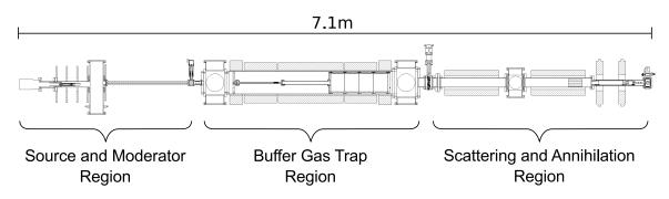
Figure 2.1: Schematic diagram of the BGT-based beamline.
