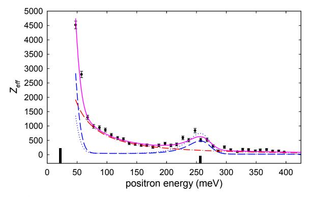
**Figure B.17**: Annihilation spectrum for bromoform (CHBr<sub>3</sub>):  $\varepsilon_b = 121 \pm 2$  meV and  $\eta = 0.07$ . Possible energy shifts present.
