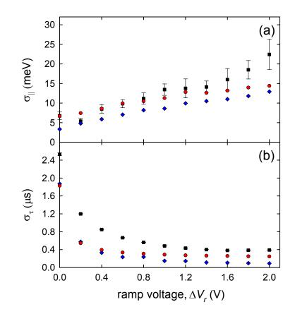
**Figure 5.6**: Effect of ramp voltage on the BGT beam. Standard deviations of the (a) parallel energy and (b) time distributions using various ramp voltages,  $\Delta V_r = V_s - V_E$ , with  $V_T = 30$  V,  $V_E = 3$  V, and  $\tau_r = 10 \,\mu$ s. (**■**) experimental measurements, (•) simulation results, and (•) simulation results without the nominal 7 mV rms electronic noise and broadened NaI detector response.
