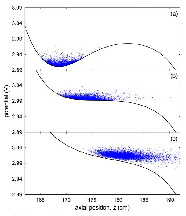
**Figure 5.2**: Simulated BGT positron ejection. (—) on-axis potential and (•) positron positions and energy at (a)  $t = 16 \ \mu$ s, (b)  $t = 18.5 \ \mu$ s and (c)  $t = 20 \ \mu$ s for the conditions described in Fig. 5.1. The ramp function is as in Eq. (2.2), with  $V_s = 3.5 \ V$ ,  $V_0 = 0 \ V$ , and  $\tau_r = 10 \ \mu$ s.
