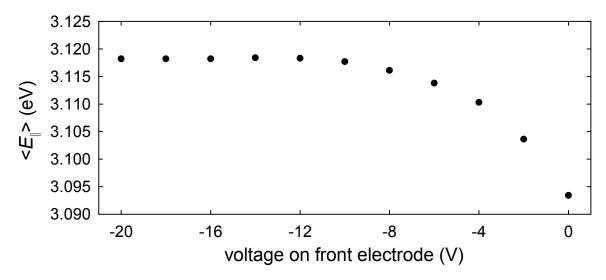
**Figure 3.10**: Effect of potential perturbations on energy. (•) measured mean parallel energy obtained as a negative voltage of various values is applied to an electrode immediately upstream of the RPA. This technique provides a measure of effects due to positive potential perturbations in the RPA potential.
