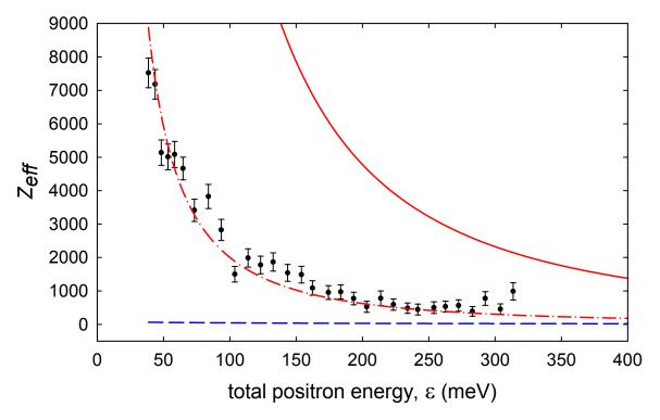
**Figure 4.3**: Annihilation spectrum for carbon tetrabromide (CBr<sub>4</sub>) [35]; (•) measured data, (--) GL model from Eq. (A.8) with  $\varepsilon_b = 115$  meV, (--) MRA model from Eq. (A.11) and (--) MRA model scaled by factor  $\eta = 0.13$ .
