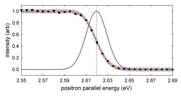
**Figure 3.2**: Measured BGT beam cumulative parallel energy distribution. (•) cumulative energy distribution measured at an RPA magnetic field of  $B \sim 650$  G ( $M \approx 1$ ), (--) EMG fit to data, and (--) negative-derivative of fit, thus representing the parallel energy distribution. Shaded areas and vertical dotted lines show the 95 % confidence interval and mean parallel energy obtained from the fit, respectively.
