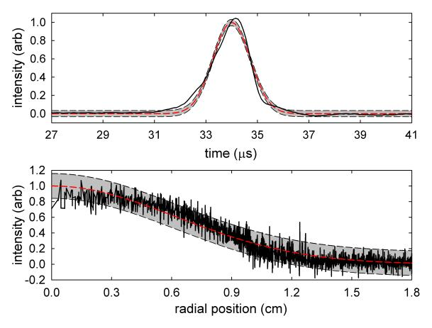
**Figure 3.5**: Beam temporal and radial distributions obtained from the BGT: (a) temporal distribution yielding  $\Delta \tau = 1.7 \ \mu$ s FWHM ( $\sigma_{\tau} = 0.71 \ \mu$ s), and (b) radial distribution yielding  $\Delta R = 1.4 \ \text{cm}$  FWHM at 320 G ( $\Delta R = 1.0 \ \text{cm}$  FWHM in ~ 650 G trap field). Shaded regions show 95 % confidence intervals estimated from the fits.
