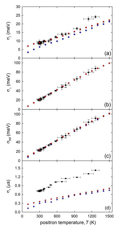
**Figure 5.7**: Effect of positron temperature on the BGT beam. Standard deviations of (a) parallel energy, (b) perpendicular energy, (c) total energy, and (d) time distributions of positron beam, generated at different initial positron temperatures: ( $\blacksquare$ ) experimental measurements; ( $\bullet$ ) simulation results and ( $\blacklozenge$ ) simulation results without the 7 mV RMS electronic noise and broadening due to NaI detector response.
