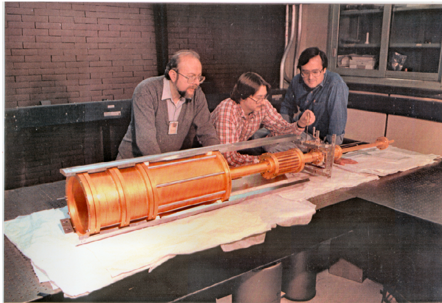
Fig. 3. Gold-plated copper electrode structure of the buffer-gas positron accumulator as assembled in 1986. From left to right, Al Passner, Fred Wysocki, and Marv Leventhal. The electrodes sit on laser tables where equipment for Allen Mills' Ps spectroscopy experiment [14] was to be set up.
