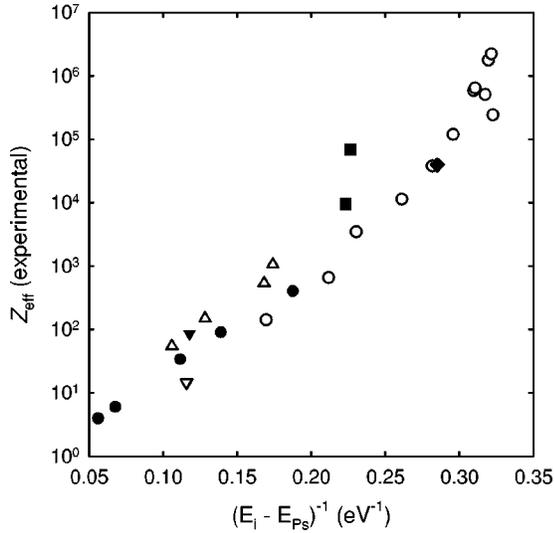
FIG. 9. Scaling of  $Z_{\text{eff}}$  with  $(E_i - E_{\text{Ps}})^{-1}$ . The data plotted are all the atoms and molecules for which physical parameters are available for calculation of the predictions of the other models discussed in Sec. VD: (●) noble gases, (▽)  $\text{H}_2$ , (solid triangle, down)  $\text{SF}_6$ , (○) alkanes, (△) perfluorinated alkanes, (solid square) perchlorinated alkanes, and (solid diamond)  $\text{CBr}_4$ .
