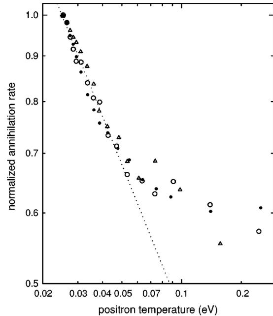
FIG. 8. Temperature dependence of the annihilation rates for methane (○), deuterated methane (△), and butane (●). The dotted line (⋯) is a fit to the lower-temperature data with the coefficient of  $-0.55$ . The theoretical fit for methane is shown in Fig. 7. The data for butane show  $1/\sqrt{T}$  behavior at small temperatures, which is characteristic of the resonant annihilation.
