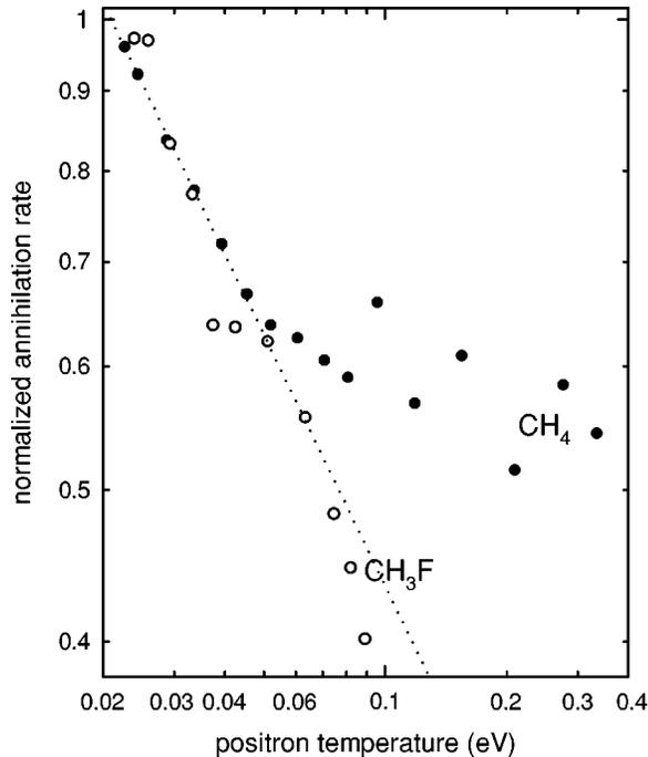
FIG. 5. Dependence of annihilation rates on positron temperature: (●) methane ( $\text{CH}_4$ ), and (○) fluoromethane ( $\text{CH}_3\text{F}$ ). The annihilation rates are normalized to their room-temperature values. The dotted line ( $\cdots$ ) is a fit to the lower-temperature data with the coefficient of  $-0.53$ .
