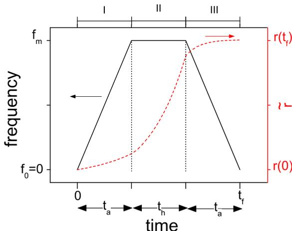
FIG. 7. Schematic diagram of the bidirectional autoresonance technique: (–) frequency, and (–) plasma radius as a function of time, where  $t_a$  is the time duration of the frequency change to or from the maximum frequency  $f_m$  and  $t_h$  is the time  $f$  is held constant.
