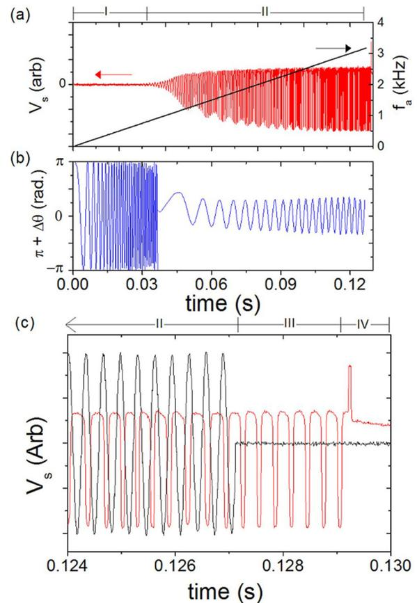
FIG. 3. (a) Pick-up signal (red line) with the autoresonant drive frequency (black line) shown for reference; (b) relative phase difference  $\phi$  between drive and pick-up signals; and (c) the drive (black line) and pick-up (red line) signals during the last few cycles as the chirp ends. Data for the short plasma with  $f_1^m \approx 1$  kHz, drive amplitude  $V_0 = 2$  V, and chirp rate  $\alpha = 25$  kHz/s. See text for details.
