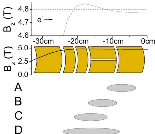
FIG. 14. (a) Expanded  $B_z$  field scale in trap region. (b) Schematic of trap electrodes with full range  $B_z$  field overlaid. (c) Plasma positions with respect to trap electrodes and  $B_z$  field.
