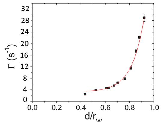
FIG. 13. Plasma expansion rate, calculated from the fits in Fig. 12, as a function of  $d/r_w$ . Also shown (–) is the fit to the data. See text for details.
