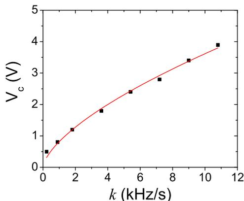
FIG. 5. Critical drive voltage to excite a typical long plasma to  $0.65 \leq d/R_w < 0.8$  for various chirp rates  $k$ . The fit (—) corresponds to  $V_c \propto k^{0.65 \pm 0.03}$ .
