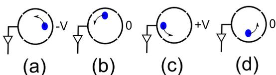
FIG. 2. Simplified schematic of plasma position (●) for four phases of the drive signal, (a) 0, (b)  $\pi/2$ , (c)  $\pi$ , and (d)  $3\pi/2$  of the applied autoresonant drive. Note the image signal is received from the segment opposite the drive.
