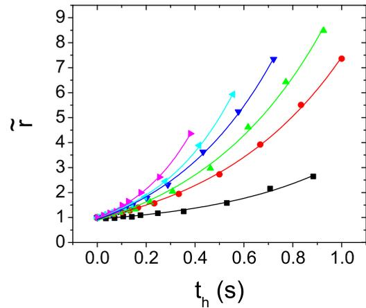
FIG. 12. Plasma radius, normalized to the radius for  $t_h = 0$ , as a function of hold time  $t_h$  at various displacements by varying  $t_a$  at constant chirp rate,  $k = 2.5$  kHz/s: (■)  $d/r_w = 0.43$ , (●)  $d/r_w = 0.52$ , (▲)  $d/r_w = 0.63$ , (▼)  $d/r_w = 0.67$ , (◀)  $d/r_w = 0.70$ , and (▶)  $d/r_w = 0.76$ . The data at each displacement (–) are fit with separate exponential functions to extract the expansion rate,  $\Gamma(d)$ .
