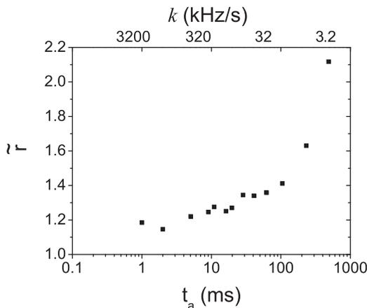
FIG. 11. Final plasma radius, at  $d_f/r_w = 0.82$ , normalized to the initial radius at  $d=0$ , as a function of the autoresonant time  $t_a$ , on a semi-logarithmic scale, for a plasma with  $L_p \sim 4$  cm.
