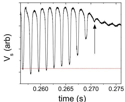
FIG. 9. Pick-up signal for a plasma excited to  $d/r_w \approx 0.8$  while the drive amplitude is still on; (–) indicates average peak amplitude for the preceding 70 ms ( $\sim 30$  cycles), highlighting that the charge is lost in the final 2–3 cycles. Arrow indicates the point of total charge loss, which is followed by pick-up from the drive signal only.
