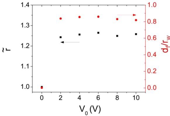
FIG. 10. (■) Variation of plasma radius (normalized to the initial radius) with drive amplitude  $V_0$ , applied for a fixed time  $t_a$  at constant chirp rate  $k$ ; and (●) the corresponding displacement  $d_f/r_w$ .
