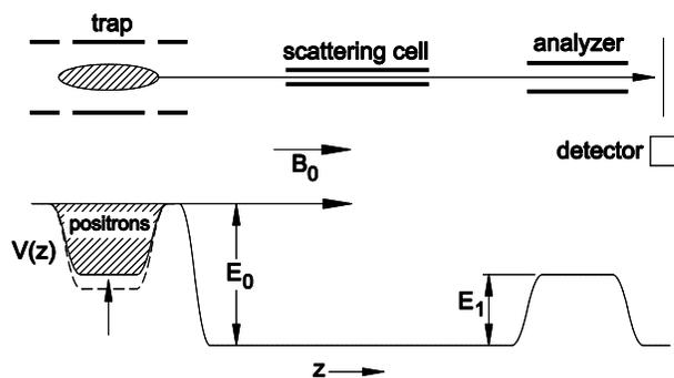
FIG. 1. (above) Schematic diagram of the scattering experiment showing the positron trap, scattering cell, and analyzer. (below) Plot of the potential profile  $V(z)$  used to form and measure a scattered positron beam. As the depth of the potential well is reduced, positrons are forced over the potential barrier creating a positron beam at energy  $E_0$  and analyzed using the retarding voltage  $E_1$ .
