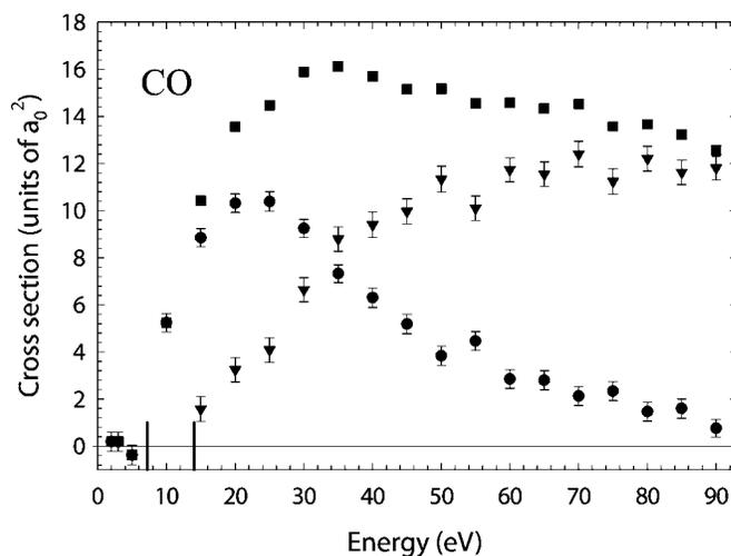
FIG. 6. Integral cross sections for CO: (●) positronium formation, (▼) direct ionization, and (■) total ionization.
