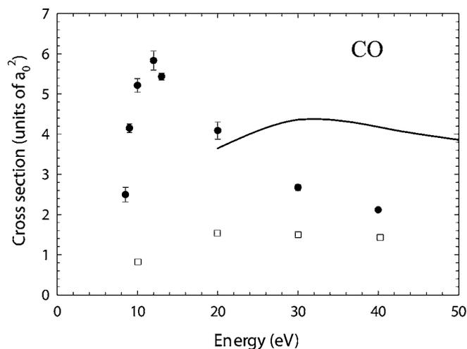
FIG. 13. Integral cross sections for the excitation of the  $A \ ^1\Pi$  state in CO by ( $\bullet$ ) positron and ( $\square$ ) electron impact [28]. Also shown ( $-$ ) is a theoretical calculation for the excitation of the  $A \ ^1\Pi$  state in CO by electrons [29].
