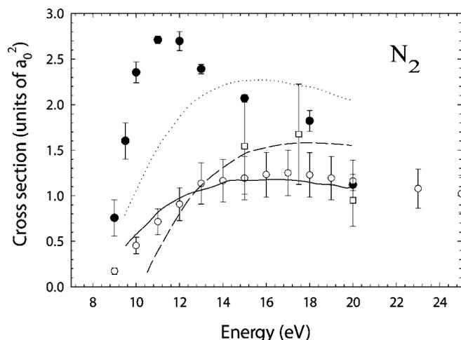
FIG. 11. Integral cross sections in N<sub>2</sub> for the excitation of the  $a^1\Pi$  states by (●) positrons and (○, □) [24,25] electrons. Also shown are the three theoretical predictions for positron excitation of the  $a^1\Pi$  state from Ref. [26]. All curves were calculated using the Schwinger multichannel formalism with different choices for the basis sets: (—) mixed antibonding orbitals, (···) mixed bonding orbitals, and (--) Hartree Fock orbitals.
