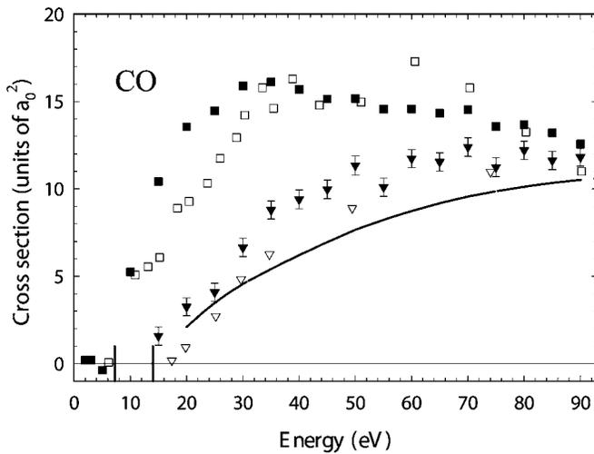
FIG. 7. Present measurements of the integral cross sections for CO: ( $\blacktriangledown$ ) direct ionization and ( $\blacksquare$ ) total ionization. Shown for comparison are the experimental results of Ref. [17] for ( $\nabla$ ) direct ionization and ( $\square$ ) total ionization and theoretical calculation (—) of Ref. [18]. Vertical bars mark the positions of the Ps formation and direct ionization thresholds.
