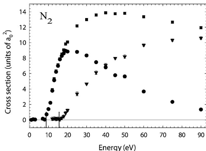
FIG. 4. Integral cross sections for  $N_2$ : (●) positronium formation, (▼) direct ionization, and (■) total ionization. Vertical bars in this and subsequent figures mark the positions of the Ps formation and direct ionization thresholds.
