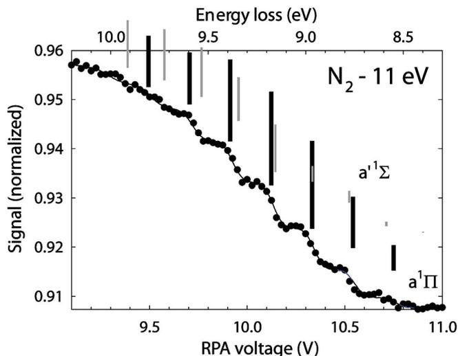
FIG. 3. (Color online) Raw data for electronic excitation in  $\text{N}_2$ . The positron energy in the scattering cell is 11 eV, and the beam transport energy (set by  $V$  in Fig. 1) is 19.3 eV. The positions of vibrational manifold energies for each electronic state are shown as vertical bars. The lengths of the bars are proportional to the Franck-Condon factor for each transition and therefore show the relative weighting of the vibrational states within an electronic state.
