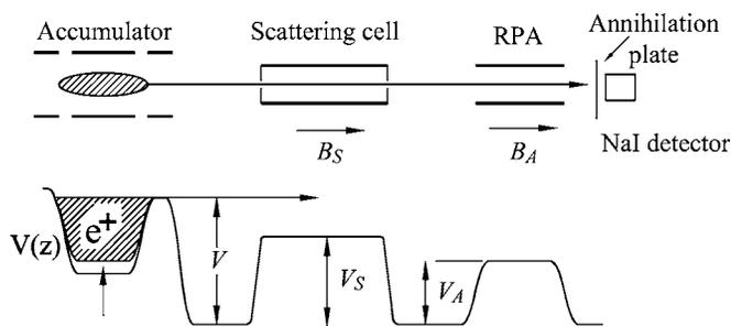
FIG. 1. Schematic diagram of the electrode structure (above) and the electric potentials (below) used to study scattering with a trap-based positron beam. The positron beam is guided by an applied magnetic field of strength  $B_S$  in the scattering cell and  $B_A$  in the retarding potential analyzer (RPA).
