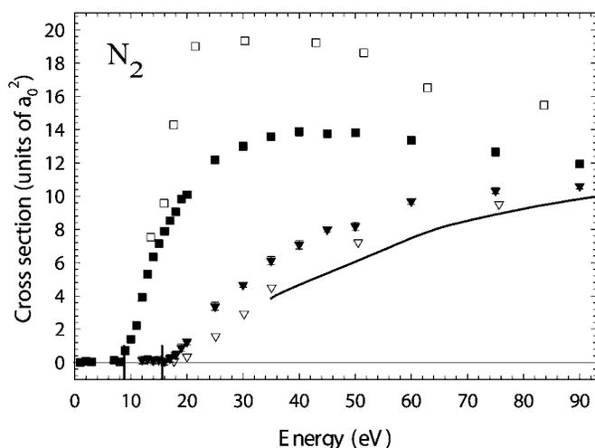
FIG. 5. Integral cross sections for  $N_2$ : (▼) direct ionization and (■) total ionization cross section. Shown for comparison are the experimental results of Ref. [16] for (▽) direct ionization and (□) total ionization. The CPE theoretical result of Ref. [2] for direct ionization is shown by the solid line.
