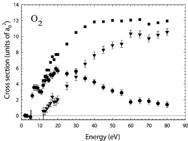
FIG. 8. Integral cross sections for  $O_2$ : ( $\bullet$ ) positronium formation, ( $\blacktriangledown$ ) direct ionization, and ( $\blacksquare$ ) total ionization.
