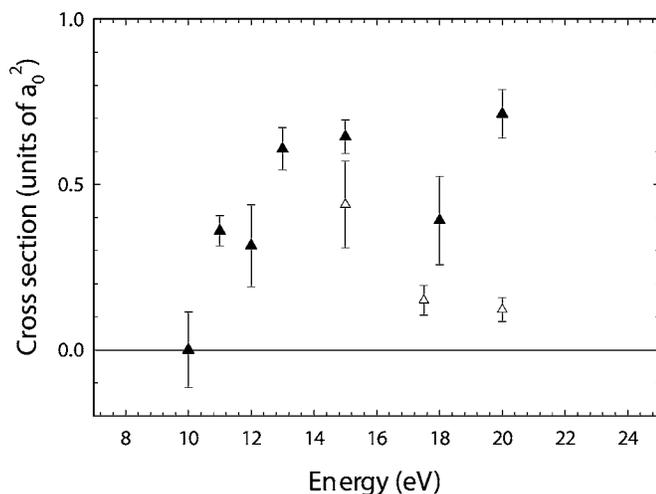
FIG. 12. Integral cross sections in  $N_2$  for the excitation of the  $a' \ ^1\Sigma$  state by ( $\blacktriangle$ ) positrons (present data) and ( $\triangle$ ) electrons (from Ref. [24]).
