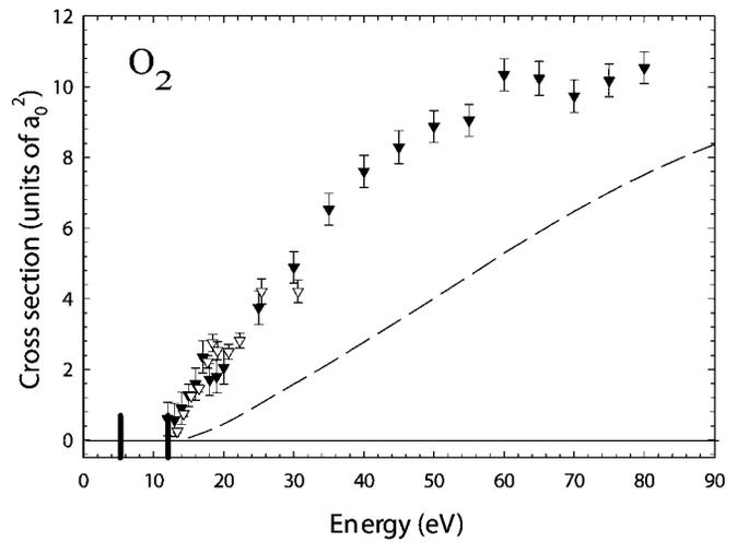
FIG. 9. Present measurements of the integral cross section for ( $\blacktriangledown$ ) direct ionization in  $O_2$ . Also shown for comparison are the experimental results of ( $\nabla$ ) [20], and the theoretical calculation of (---) [3]. Vertical bars mark the positions of the Ps formation and direct ionization thresholds.
