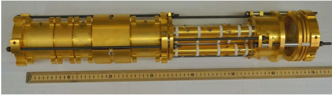
FIGURE 9. Electrode structure as built.
