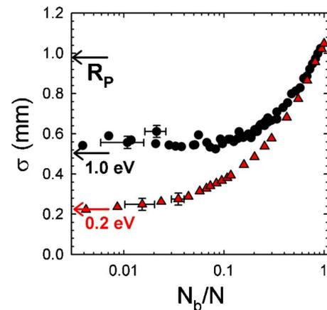
FIG. 4. (Color online) Measured beamwidths  $\sigma$  as a function of the fraction of particles,  $\beta = N_b/N$ , extracted from a (●) 1 eV and a (△) 0.2 eV plasma with  $N = 4 \times 10^8$  electrons. Sample radial profiles are shown in Fig. 2. Arrows mark  $\sigma = 2\lambda_D$  and the plasma radius.
