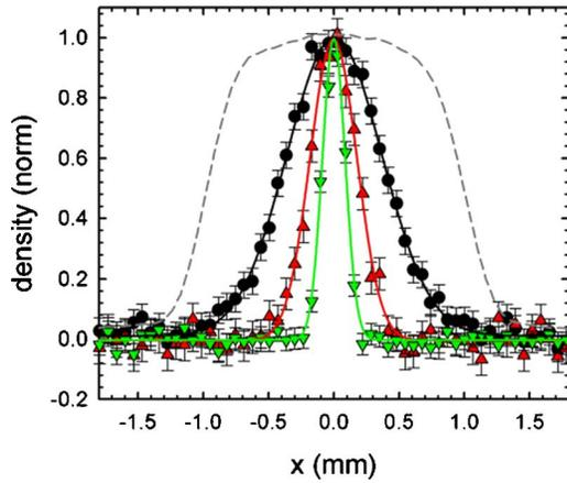
FIG. 2. (Color online) Normalized areal density profiles of beams extracted from an electron plasma with  $n=1 \times 10^9 \text{ cm}^{-3}$  at temperatures of (●) 1.0, (△) 0.2, and (▽) 0.04 eV. Solid lines are Gaussian fits, as described by Eq. (2). The dashed line is the areal density of the initial plasma.
