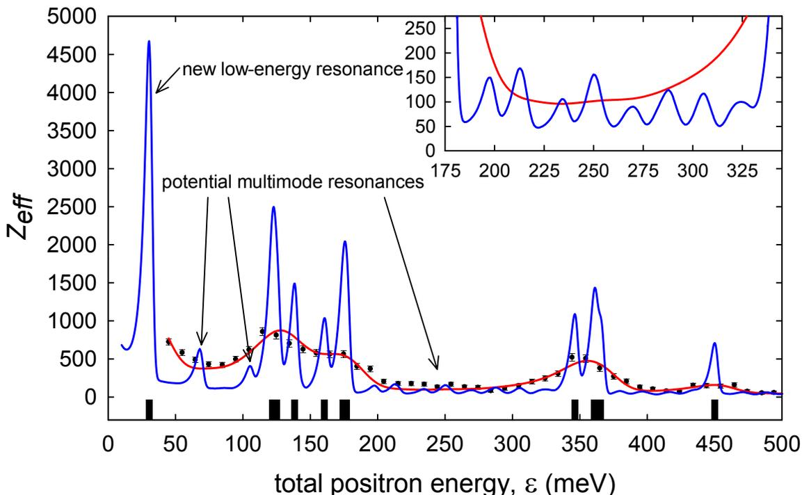
**Figure 7.10:** BGT vs. CBT annihilation spectrum for methanol ( $\text{CH}_3\text{OH}$ ): ( $\bullet$ ) measured  $Z_{\text{eff}}$ , ( $—$ ) total model from Eq. (A.16) fit to data with BGT beam distribution (cf. Table B.12), and ( $—$ ) total model using same fit parameters but with CBT beam distribution. Vertical bars show vibrational mode energies downshifted by binding energy. Inset shows low  $Z_{\text{eff}}$  resonance in more detail.
