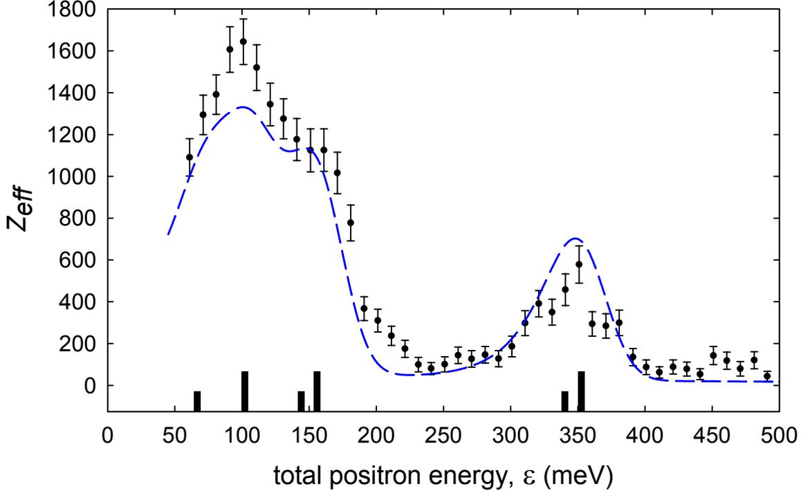
**Figure 4.1:** Annihilation spectrum for methyl chloride ( $\text{CH}_3\text{Cl}$ ) [33]; ( $\bullet$ ) measured data and ( $- -$ ) GL model from Eq. (A.8) with  $\epsilon_b = 24$  meV. Vertical bar positions represent vibrational mode energies downshifted by the binding energy and heights represent mode degeneracies.
