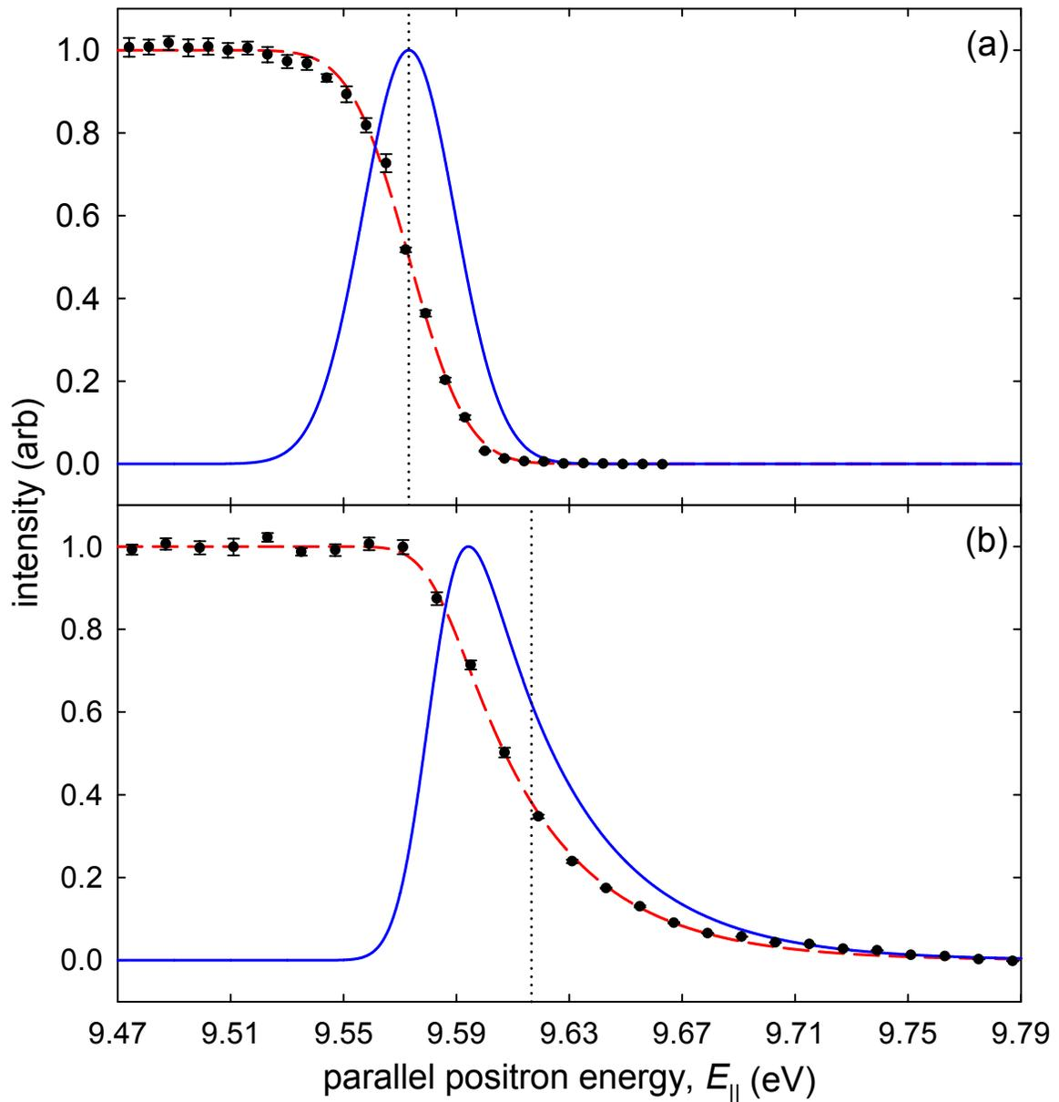
**Figure 6.1:** Example cutoffs used to obtain positron temperature. Parallel energy distribution measured at (a)  $B \sim 800$  G, and (b)  $B' \sim 200$  G; ( $\bullet$ ) measured integrated parallel energy distributions, ( $- -$ ) fits to data, and ( $-$ ) derivatives of fits that represent the positron energy distributions. Dotted vertical lines represent fitted mean parallel energies  $\bar{E}_{\parallel}$  and  $\bar{E}'_{\parallel}$ .
