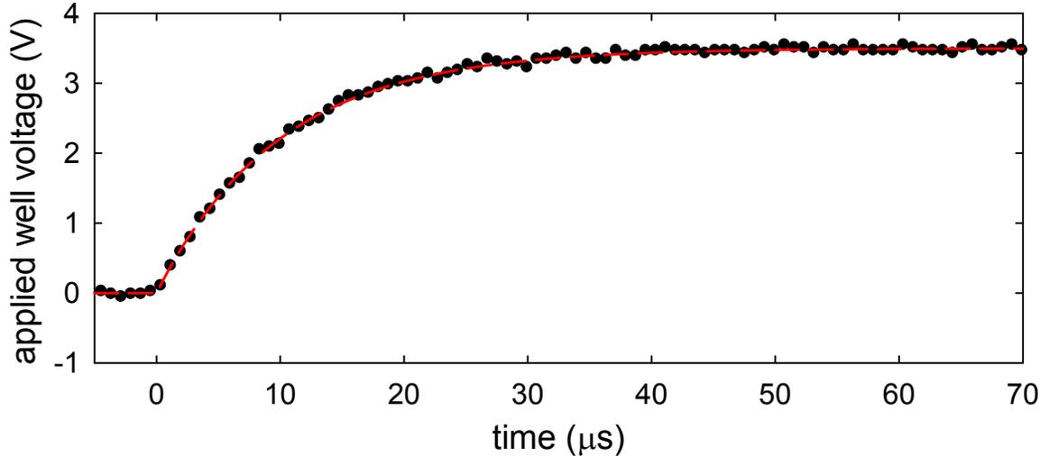
**Figure 2.6:** Typical BGT ejection ramp function. (•) applied voltage as measured on an oscilloscope, and (---) Eq. (2.2) with  $V_s = 3.5$  V,  $V_0 = 0$  V and  $\tau_r = 10$   $\mu$ s.
