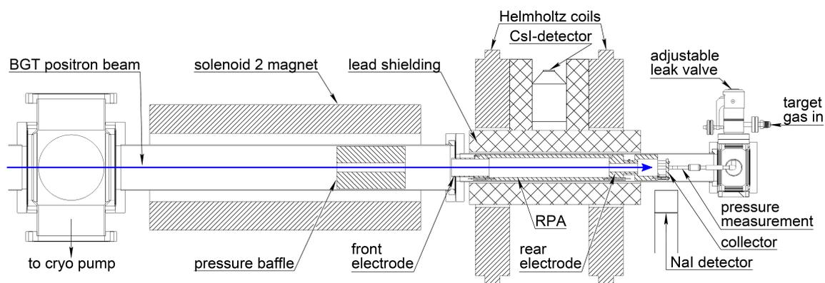
**Figure 2.8:** Schematic diagram of the annihilation region. A solenoidal magnet and a set of Helmholtz coils provide a magnetic field which varies between 500 and 700 G, while the front and rear electrodes, the RPA, collector and NaI gamma-ray detector are used to diagnose the BGT beam. The leak valve, pressure baffle, lead shielding, and CsI gamma-ray detector are used for positron annihilation studies.
