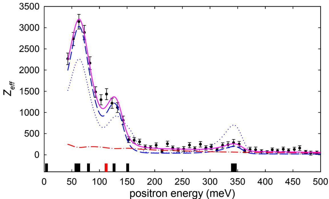
**Figure B.5:** Annihilation spectrum for dichloromethane ( $\text{CH}_2\text{Cl}_2$ ):  $\varepsilon_b = 31 \pm 1$  meV and  $\eta = 0.28$ .
