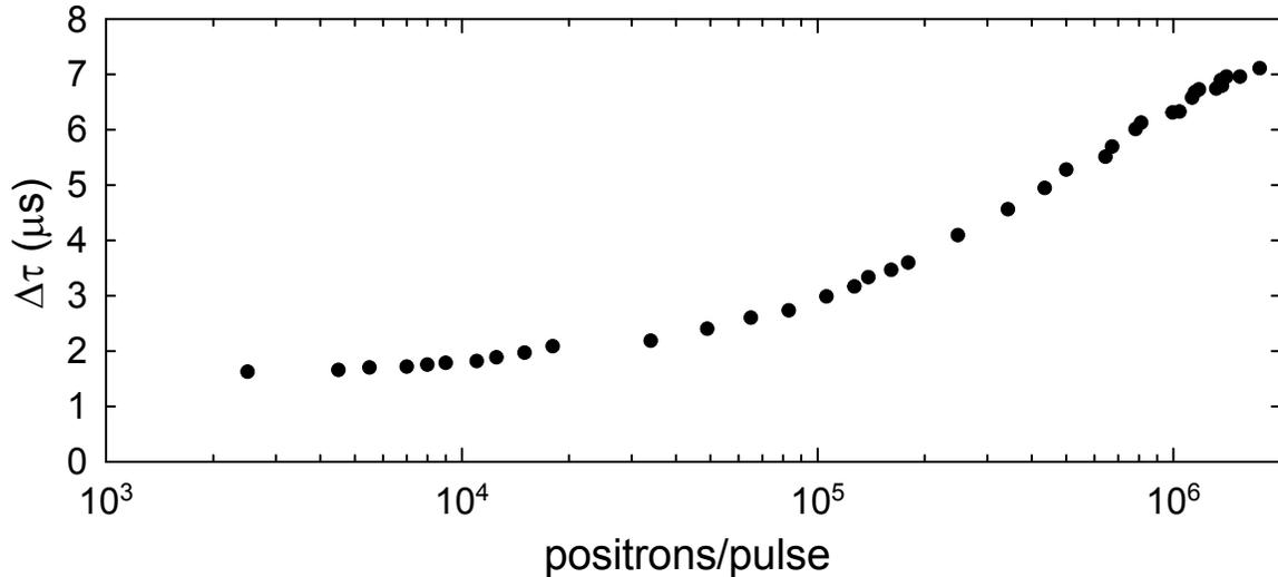
**Figure 3.7:** BGT temporal spread dependence on positrons number.
