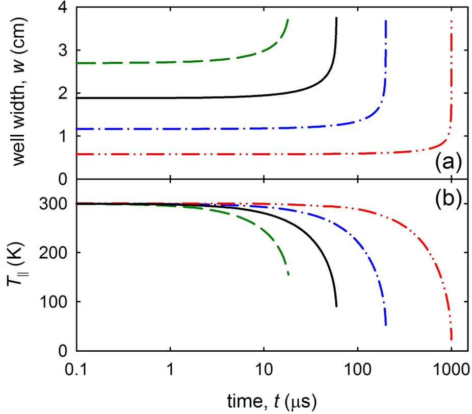
**Figure 5.13:** Effect of well depth on beam formation. (a) average potential well width as seen by the particles and (b) particle parallel temperature as a function of time obtained from the simulation using an initial well depth of ( $- -$ ) 1 V, ( $-$ ) 3 V, ( $- \cdot -$ ) 10 V and ( $- \cdot \cdot -$ ) 50 V.
