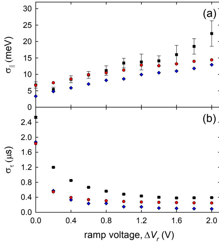
**Figure 5.6:** Effect of ramp voltage on the BGT beam. Standard deviations of the (a) parallel energy and (b) time distributions using various ramp voltages,  $\Delta V_r = V_s - V_E$ , with  $V_T = 30$  V,  $V_E = 3$  V, and  $\tau_r = 10$   $\mu$ s. (■) experimental measurements, (●) simulation results, and (◆) simulation results without the nominal 7 mV rms electronic noise and broadened NaI detector response.
