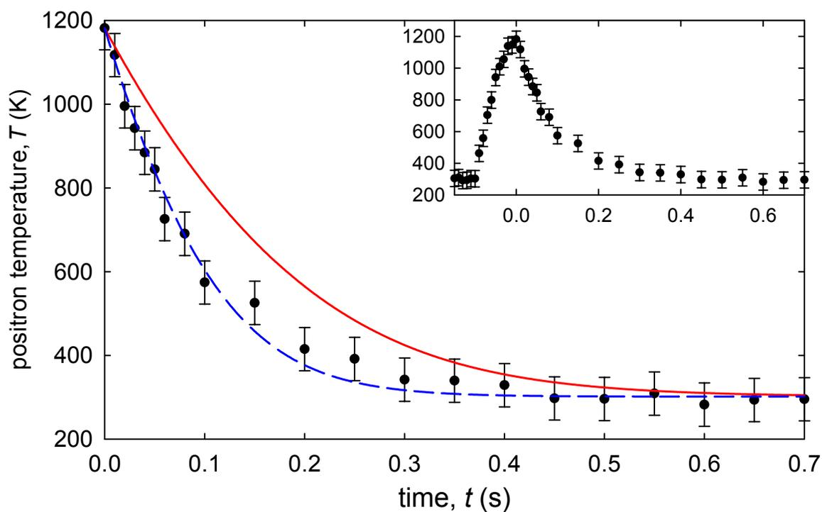
**Figure 6.3:** Positron cooling using  $15 \pm 1.5 \mu\text{torr}$  of  $\text{N}_2$  at 300 K: ( $\bullet$ ) measured data; ( $—$ ) solution to Eq. (6.7) for quadrupole rotational excitation and de-excitation of all contributing  $j$  rotational states; and ( $- -$ ) solution to Eq. (6.7) with cross sections scaled up by  $\eta = 1.8$ . The inset shows the full heating and cooling cycle.
