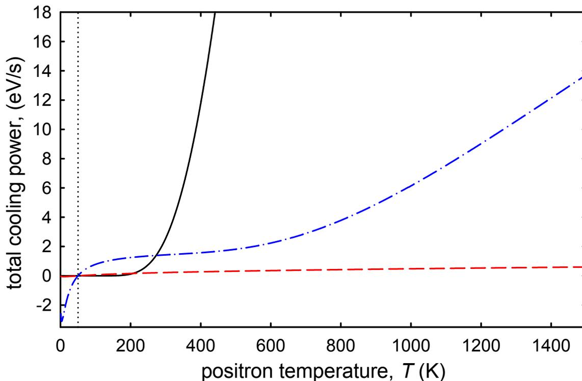
**Figure 6.8:** ositron cooling power at 50 K. Calculated total cooling power, defined as in Eq. (6.6), for the conditions described in Fig. 6.7 for (—)  $\text{CF}_4$ , (- -)  $\text{N}_2$  and (- · -)  $\text{CO}$ . Vertical dotted line shows gas temperature. See text for details.
