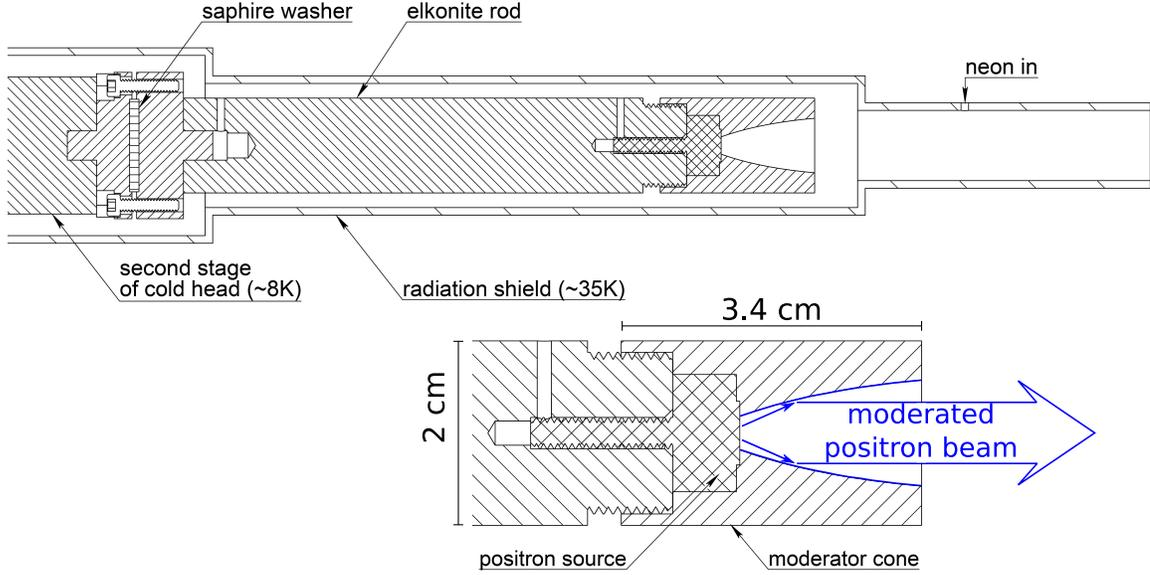
**Figure 2.2:** Schematic diagram of the source and moderator assembly. The  $^{22}\text{Na}$  source and copper moderator cone are attached through an elkonite rod to the second-stage of a two-stage cryocooler which is maintained at 8 K. The assembly is surrounded by a radiation shield which is attached to the first-stage of the cryocooler and maintained at  $\sim 35$  K.
