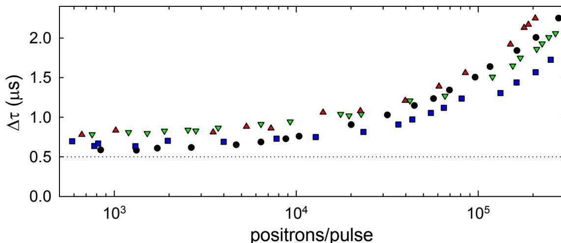
**Figure 7.9:** CBT temporal spread dependence on positrons number. (●) measured FWHM of the temporal distribution obtained as the number of positrons per pulse is varied. (▲) CBT at 300 K, radial compression on, (▼) CBT at 300 K, radial compression off, (●) CBT at 50 K, radial compression on, (■) CBT at 50 K, radial compression off. Dotted line shows minimum detector response ( $\sim 0.5 \mu\text{s}$  FWHM).
