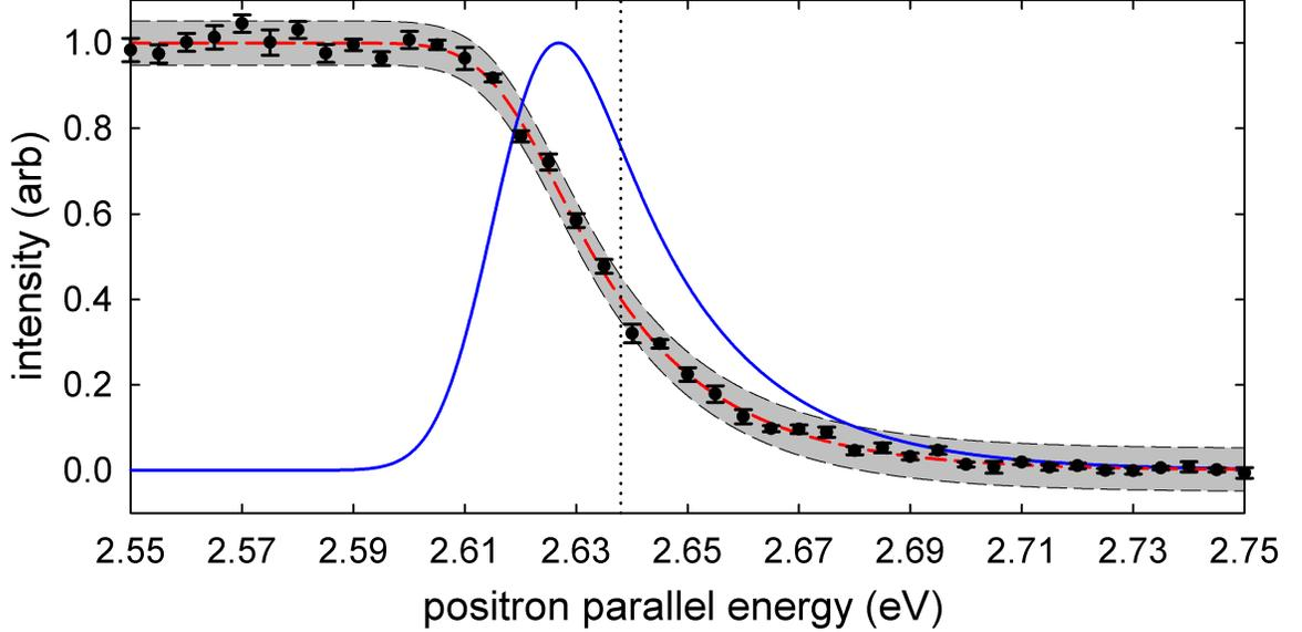
**Figure 3.3:** Measured BGT beam cumulative total energy distribution. (•) cumulative energy distribution measured at an RPA magnetic field of  $B \sim 20$  G ( $M \approx 1/30$ ), (—) EMG fit to data (Eq. (3.14)). Measurements are at a sufficiently reduced field to effectively provide a measure of the total energy distribution. Shaded areas and vertical dotted lines show the 95 % confidence interval and mean parallel energy obtained from the fit.
