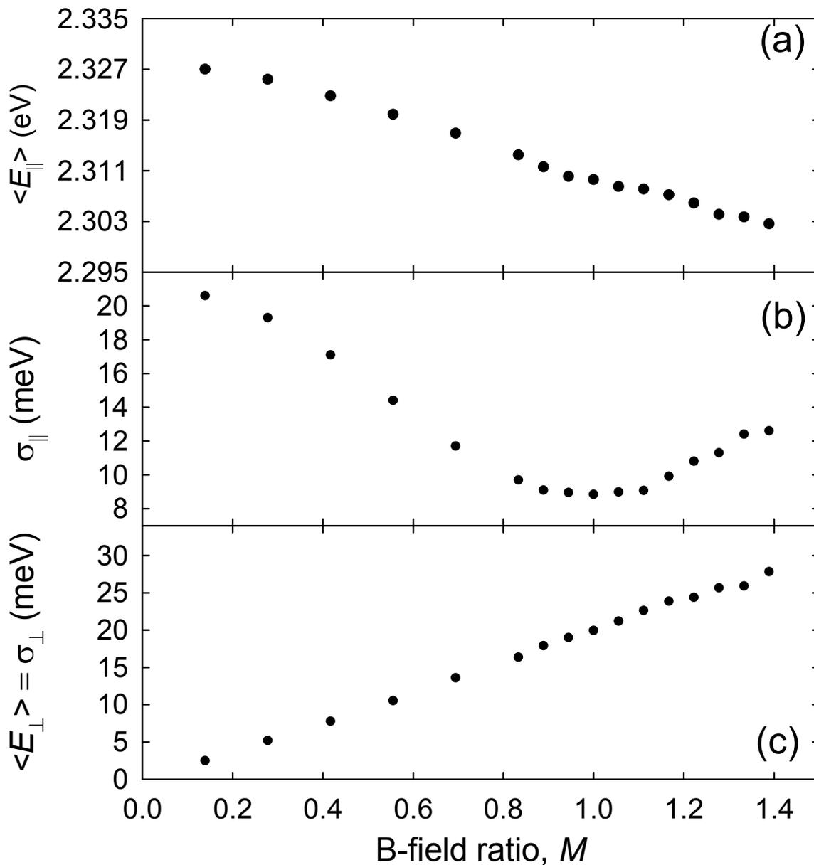
**Figure 3.6:** BGT beam measurements at various magnetic field ratios. (a) mean parallel energy, (b) standard deviation of the parallel energy distribution, and (c) mean perpendicular energy (calculated using Eq. (3.20)) at various magnetic field ratios,  $M = B_{RPA}/B_{BGT}$ . Note that, for the case of a MB perpendicular distribution,  $\bar{E}_{\perp} = \sigma_{\perp}$ .
