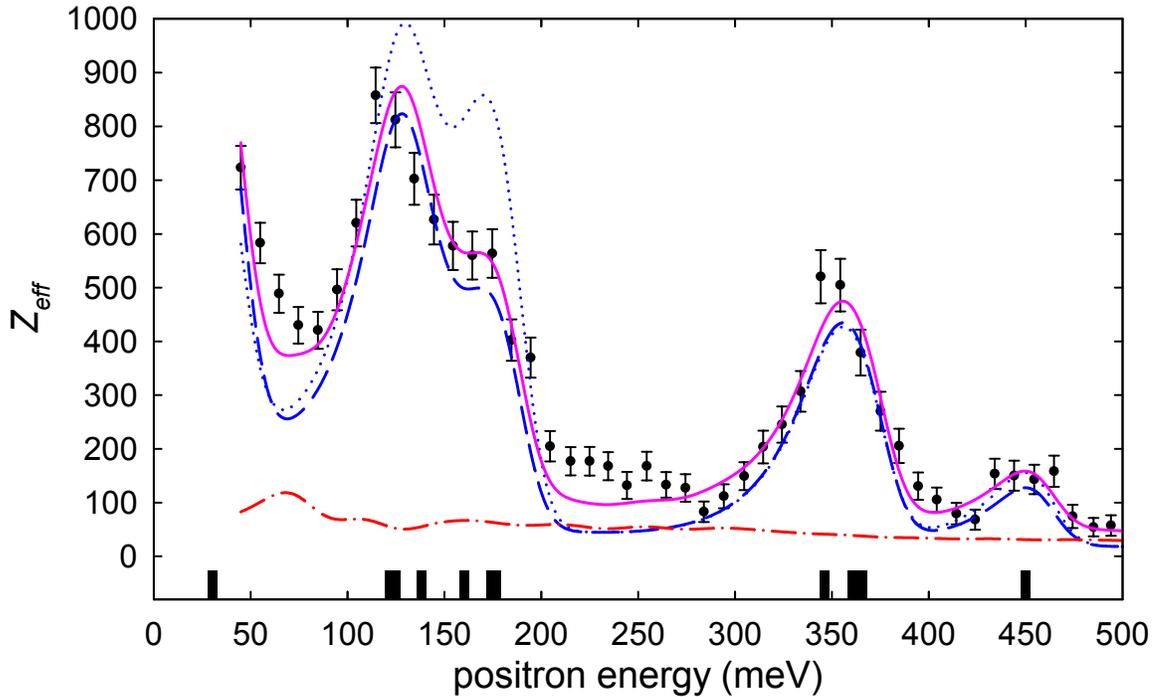
**Figure B.11:** Annihilation spectrum for methanol ( $\text{CH}_3\text{OH}$ ):  $\varepsilon_b = 6 \pm 1$  meV and  $\eta = 0.51$ . Data shown here represent new measurements. Original measurements are shown in Ref. [80].
