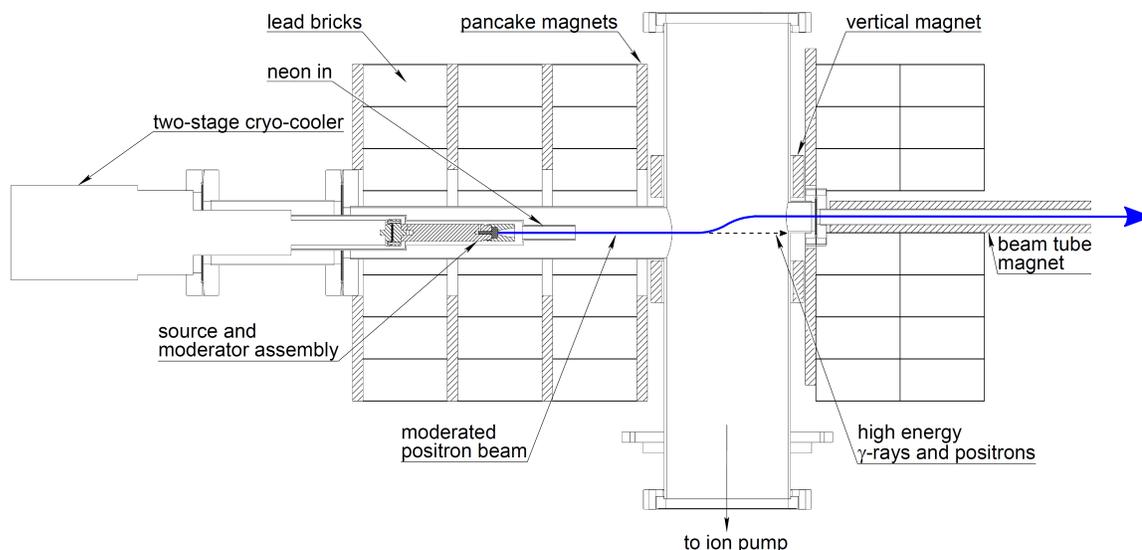
**Figure 2.3:** Schematic diagram of the source and moderator region. The source is vertically offset from the beam tube magnet to break line-of-sight with the downstream beamline. A series of pancake magnets generate a  $\sim 150$  G magnetic field for radial confinement of the moderated positrons, while a vertical coil re-aligns the beam with the downstream axis.
