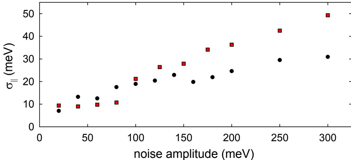
**Figure 3.9:** Effect of electronic noise on measured parallel energy distribution. Measured standard deviation of the parallel energy distribution as Gaussian noise is applied to the (●) exit-gate and (■) RPA. The horizontal axis is the peak-to-peak noise amplitude, as measured on an oscilloscope.
