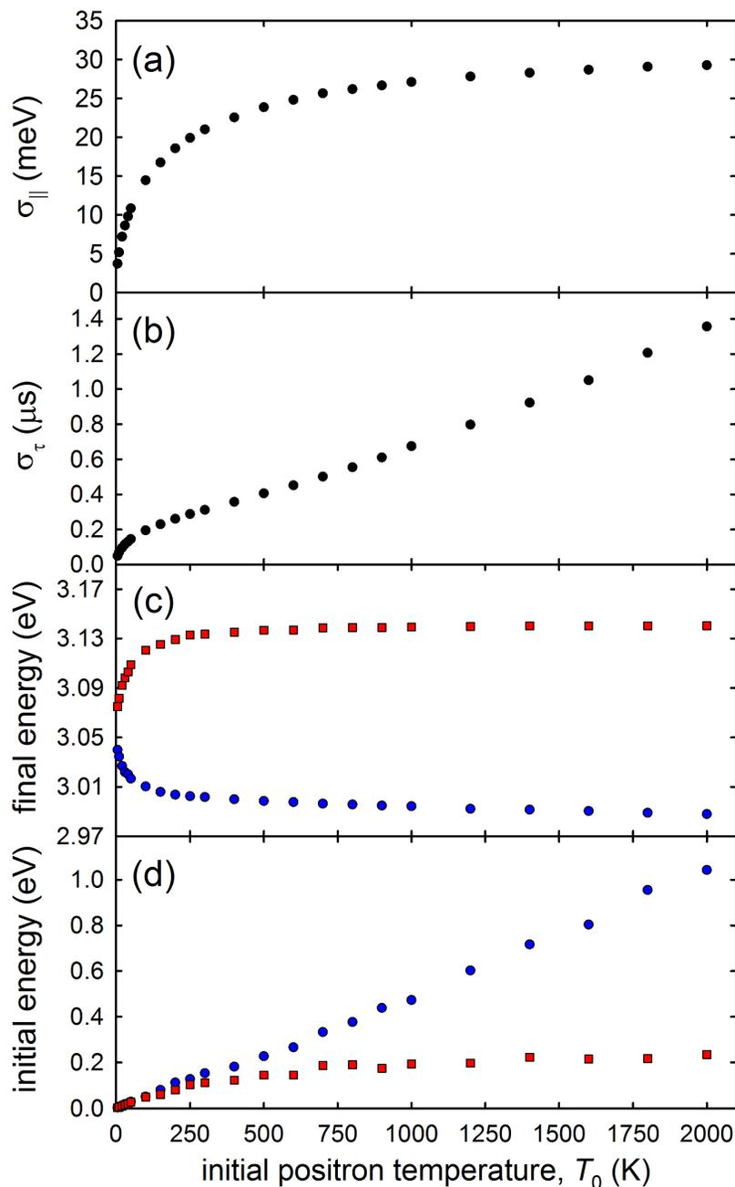
**Figure 5.11:** Effect of positron temperature on simulated beam. Standard deviations of the (a) parallel energy and (b) temporal distributions obtained from the simulation of beams generated using various initial particle temperatures. Also shown is the (c) final and (d) initial parallel energies of the particles which are ejected with the (●) lowest and (■) highest final parallel energies in the beam. All other parameters as in Fig. 5.8.
