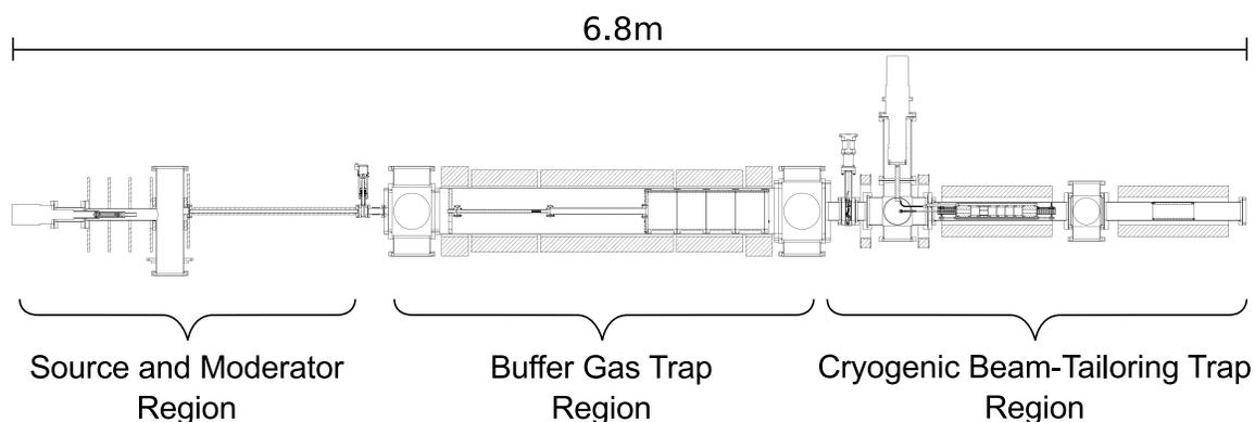
**Figure 7.1:** Schematic diagram of the CBT-based beamline. A steady-state positron beam is produced in the source and moderator region and guided into the buffer gas trap region, where it is converted into a high resolution pulsed beam. This pulsed beam is then guided into the cryogenic beam-tailoring trap region, where it is further tailored into a pulsed beam with superior characteristics.
