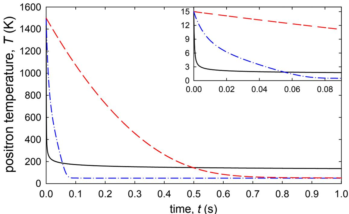
**Figure 6.7:** Positron cooling comparisons at 50 K. Solutions to Eq. (6.7) for a gas pressure of  $1 \mu\text{Torr}$  and a temperature of 50 K using cross sections scaled by the empirically determined scale factors,  $\eta$ , listed in Table 6.1 for (—)  $\text{CF}_4$ , (---)  $\text{N}_2$  and (-·-)  $\text{CO}$ . Inset shows  $\text{CF}_4$  and  $\text{CO}$  curves in more detail. See text for details.
