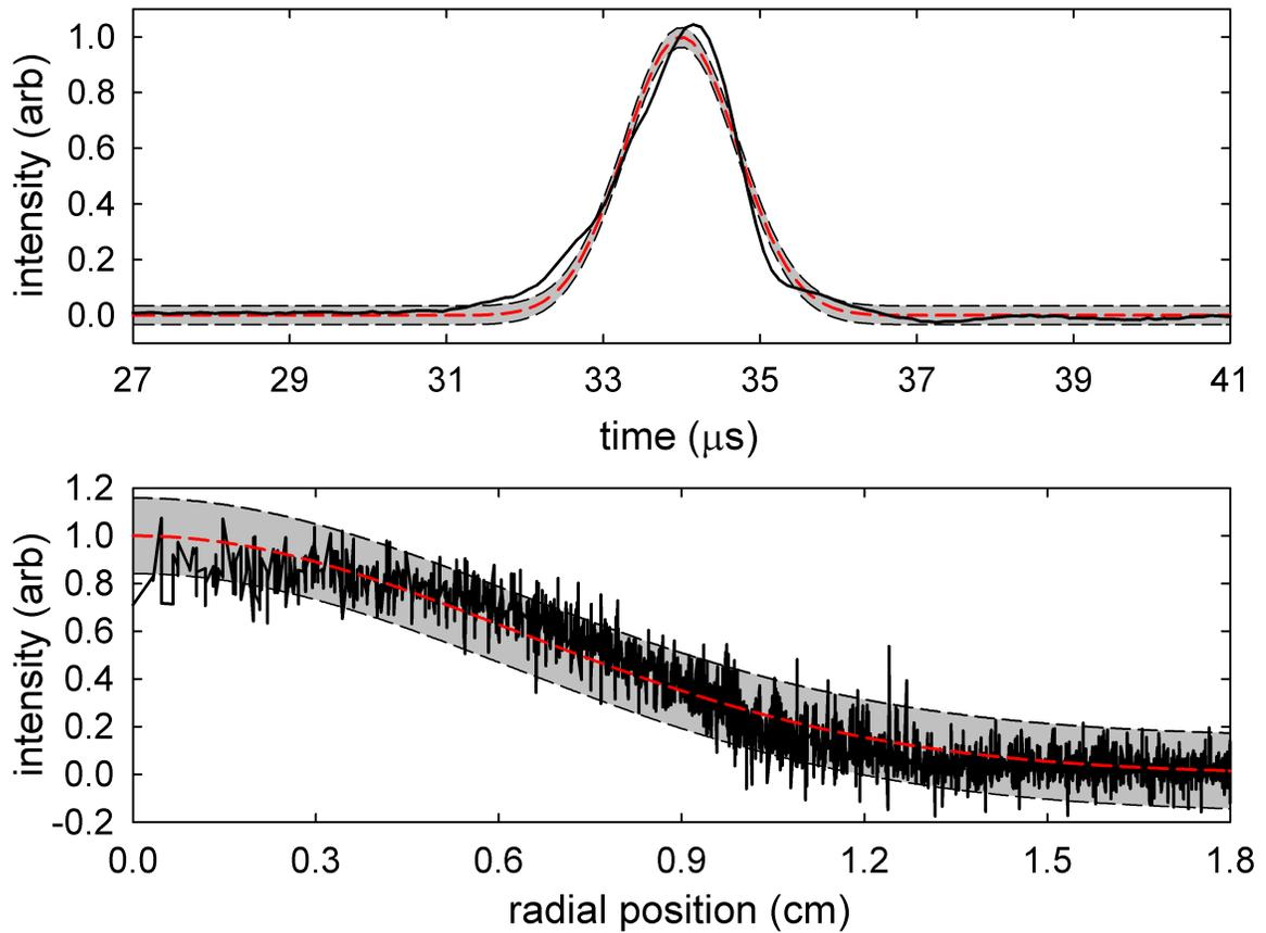
**Figure 3.5:** Beam temporal and radial distributions obtained from the BGT: (a) temporal distribution yielding  $\Delta\tau = 1.7 \mu\text{s}$  FWHM ( $\sigma_\tau = 0.71 \mu\text{s}$ ), and (b) radial distribution yielding  $\Delta R = 1.4 \text{ cm}$  FWHM at 320 G ( $\Delta R = 1.0 \text{ cm}$  FWHM in  $\sim 650 \text{ G}$  trap field). Shaded regions show 95 % confidence intervals estimated from the fits.
