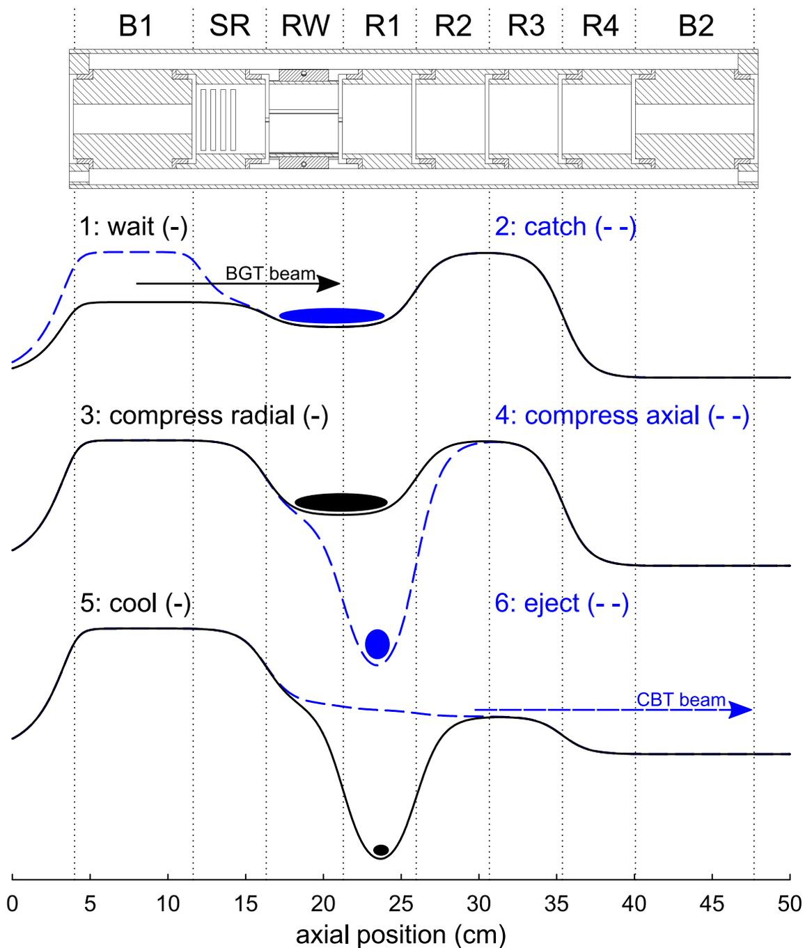
**Figure 7.4:** Schematic diagram of the CBT electrodes and potentials produced during each of its six phases of beam formation. Electrodes from left to right are the baffle B1, slotted ring SR, rotating wall RW, cylindrical rings R1 - R4, and baffle B2. Phases are labeled according to the order in which they proceed, (—) shows phases 1,3 and 5 and (---) shows phases 2,4 and 6. Shaded regions and arrows represent the positrons in the various phases. See text for details.
