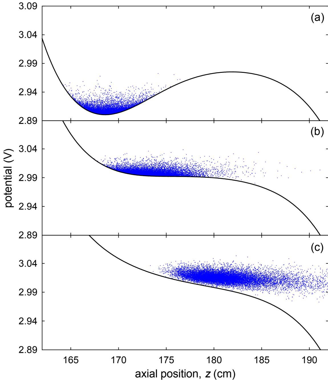
**Figure 5.2:** Simulated BGT positron ejection. (—) on-axis potential and (•) positron positions and energy at (a)  $t = 16 \mu\text{s}$ , (b)  $t = 18.5 \mu\text{s}$  and (c)  $t = 20 \mu\text{s}$  for the conditions described in Fig. 5.1. The ramp function is as in Eq. (2.2), with  $V_s = 3.5$  V,  $V_0 = 0$  V, and  $\tau_r = 10 \mu\text{s}$ .
