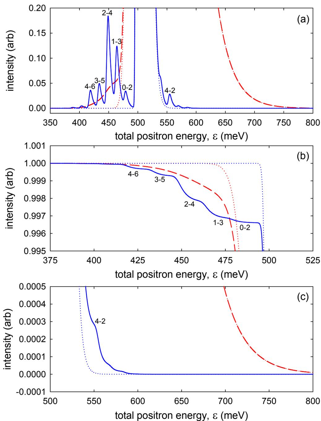
**Figure 7.14:** Simulated results of  $D_2$  rotational scattering: (a) scattered beam distributions from Eq. (7.1); (b) and (c) show integrated scattered beam distributions, thus replicating experimental measurement. (---) results using BGT beam distribution and (—) results using CBT beam distribution. Dotted curves show un-scattered beam distributions. Labels show initial and final  $j$  state. See text for details.
