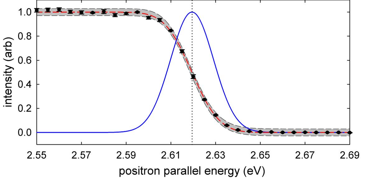
**Figure 3.2:** Measured BGT beam cumulative parallel energy distribution. (•) cumulative energy distribution measured at an RPA magnetic field of  $B \sim 650$  G ( $M \approx 1$ ), (— —) EMG fit to data, and (—) negative-derivative of fit, thus representing the parallel energy distribution. Shaded areas and vertical dotted lines show the 95 % confidence interval and mean parallel energy obtained from the fit, respectively.
