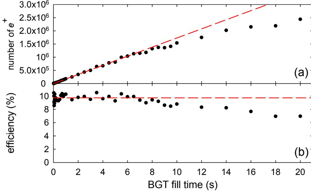
**Figure 2.5:** Typical BGT fill parameters, where (a) is the number of positrons accumulated and (b) is the trapping efficiency obtained using various BGT fill times. Red dashed lines show (a) linear fit to data and (b) mean trapping efficiency below  $\sim 6$ s.
