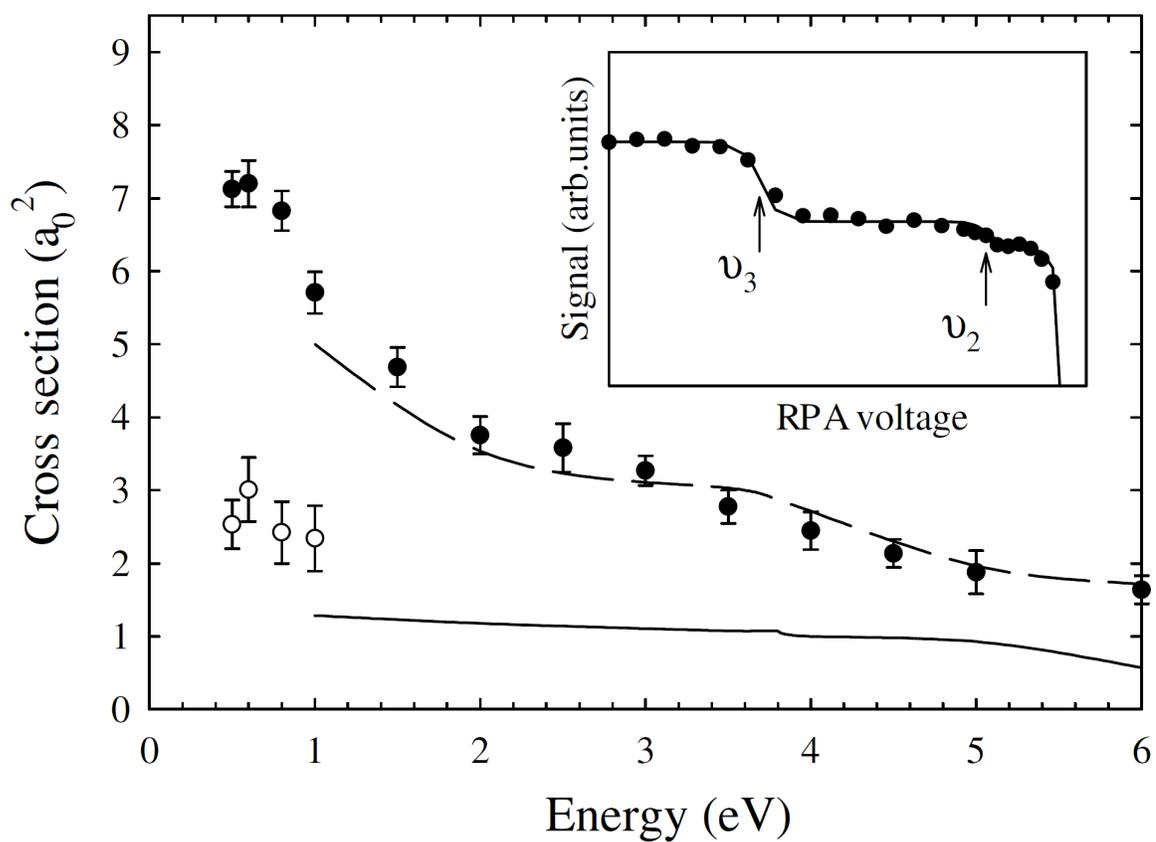
**Figure 4.5:** Cross section for excitation of the  $v_2$  and  $v_3$  vibrational modes of  $\text{CO}_2$  from Ref. [16]. ( $\circ$ ) and ( $\bullet$ ) are experimental data for the  $v_2$  and  $v_3$  modes, respectively. (—) and (---) are theory from Kimura *et al.* [42] for the same two modes. Inset shows raw RPA data, showing steps due to both vibrational modes, with the solid line showing the fitted curve.
