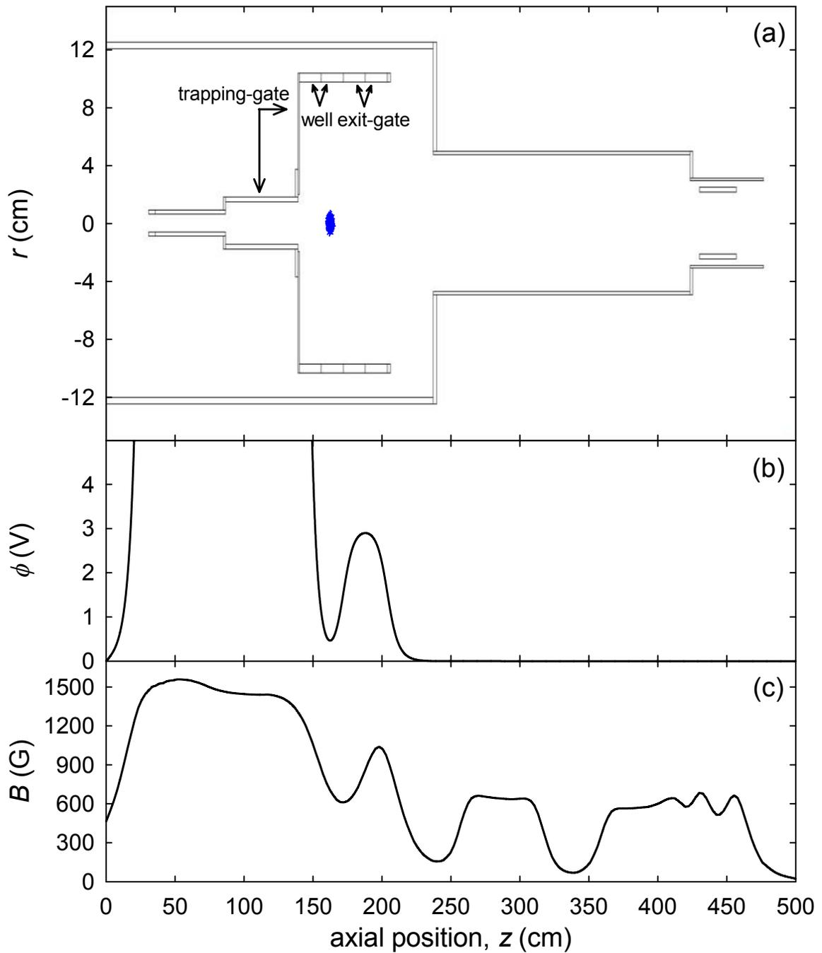
**Figure 5.1:** BGT-based beamline simulation initial conditions. (a) electrode geometry with (•) positron initial axial and radial positions, (b) initial on-axis potential and (c) axial magnetic field. For this example, the trapping-gate, well and exit-gate electrodes are set to 30, 0 and 3 V respectively.
