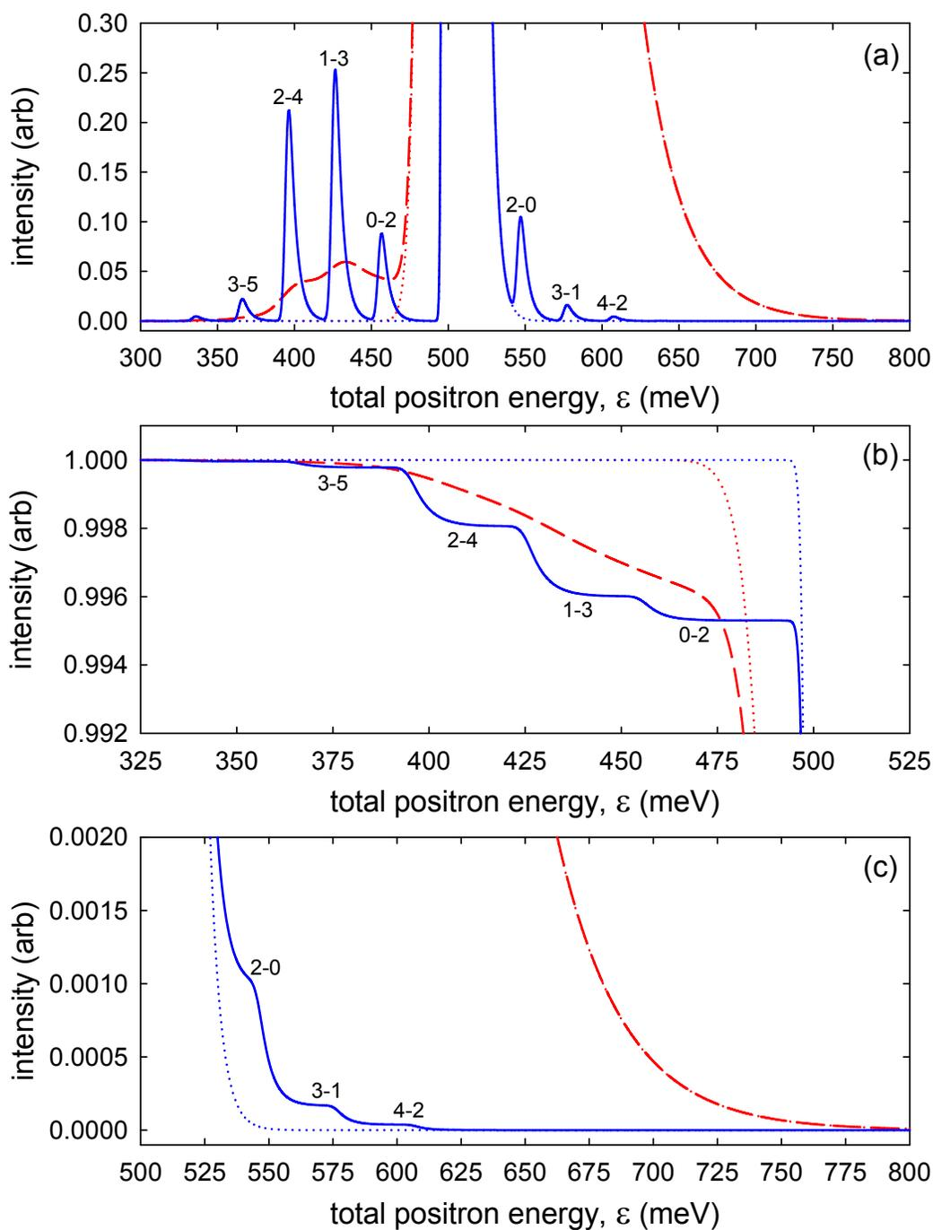
**Figure 7.13:** Simulated results of H<sub>2</sub> rotational scattering: (a) scattered beam distributions from Eq. (7.1); (b) and (c) show integrated scattered beam distributions, thus replicating experimental measurement. (—) results using BGT beam distribution and (—) results using CBT beam distribution. Dotted curves show un-scattered beam distributions. Labels show initial and final  $j$  state. See text for details.
