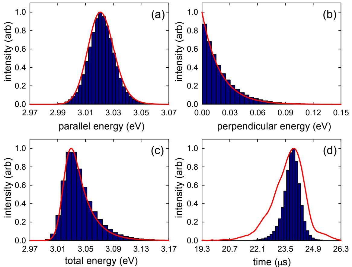
**Figure 5.5:** BGT distributions obtained from experiment and simulation for the conditions described by Figs. 5.1-5.4. (a) parallel energy, (b) perpendicular energy, (c) total energy, and (d) time. Blue bars represent simulation results, and red lines show experimental measurements. See text for details.
