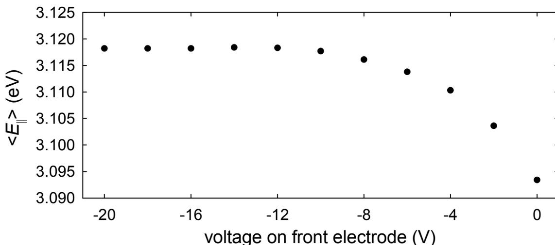
**Figure 3.10:** Effect of potential perturbations on energy. (●) measured mean parallel energy obtained as a negative voltage of various values is applied to an electrode immediately upstream of the RPA. This technique provides a measure of effects due to positive potential perturbations in the RPA potential.
