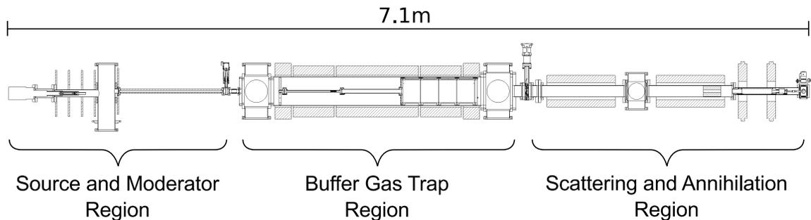
**Figure 2.1:** Schematic diagram of the BGT-based beamline.
