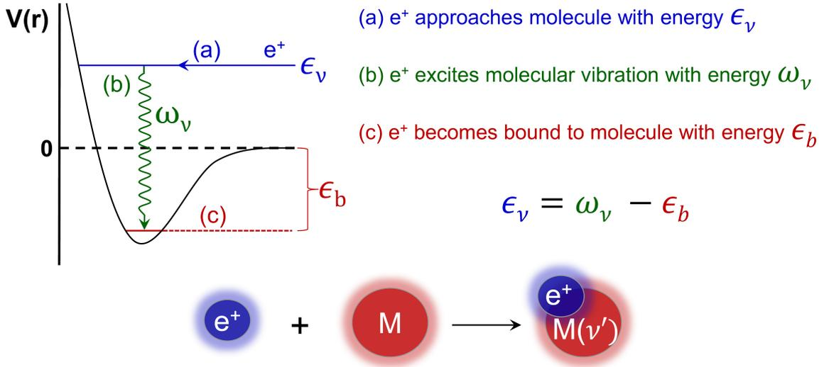
**Figure A.2:** Overview of the vibrational Feshbach resonance and positron attachment. The positron approaches the molecule with an energy  $\epsilon_v$  and excites a molecular vibration of energy  $\omega_v$ , forming a (temporary) positron-molecule bound state with binding energy  $\epsilon_b$ .
