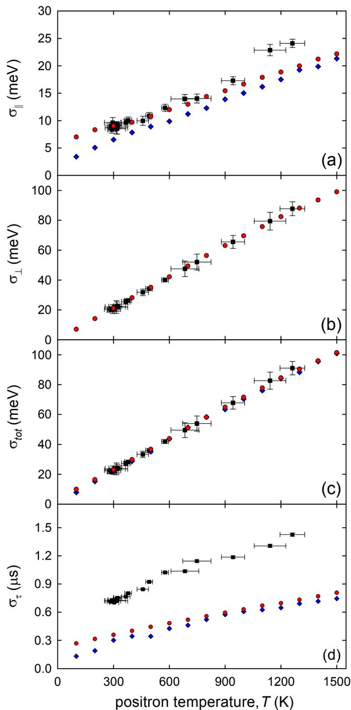
**Figure 5.7:** Effect of positron temperature on the BGT beam. Standard deviations of (a) parallel energy, (b) perpendicular energy, (c) total energy, and (d) time distributions of positron beam, generated at different initial positron temperatures: (■) experimental measurements; (●) simulation results and (◆) simulation results without the 7 mV RMS electronic noise and broadening due to NaI detector response.
