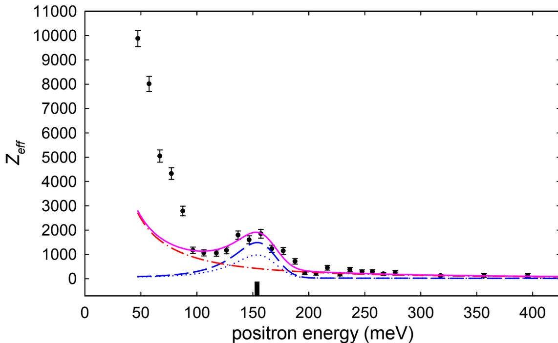
**Figure B.18:** Annihilation spectrum for bromoform-d ( $\text{CDBr}_3$ ):  $\varepsilon_b = 125 \pm 10$  meV and  $\eta = 0.07$ . Possible energy shifts present.
