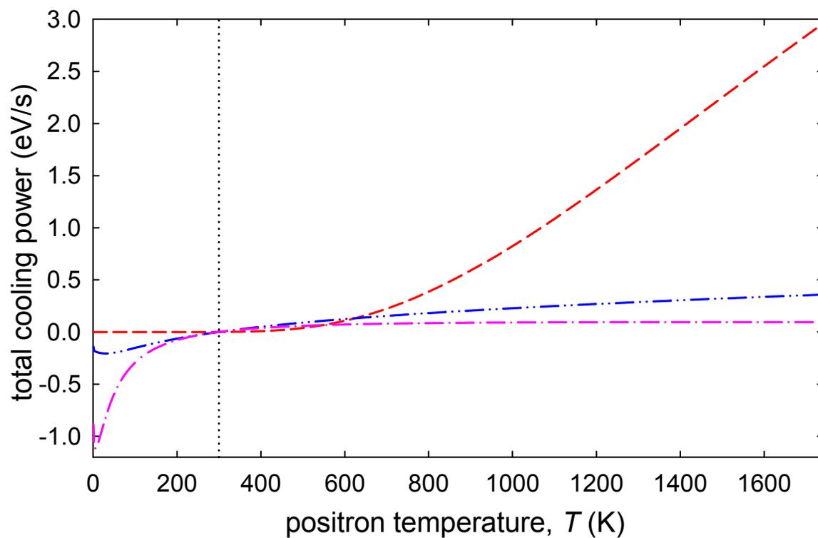
**Figure 6.5:** Positron-CO cooling power per channel. Total cooling power [defined in Eq. (6.6)] as a function of the positron temperature for  $1.74 \mu\text{Torr}$  of CO at a gas temperature of 300 K (vertical dotted line) for (---) vibrational excitation, (-·-) dipole coupled rotations and (-·-) quadrupole coupled rotations.
