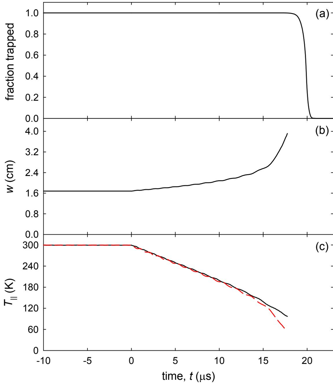
**Figure 5.3:** Simulated BGT parameters during ejection. (a) fraction of positrons remaining in the trap, (b) average width  $w$  of the potential well as seen by the positrons and (c) parallel positron temperature for the conditions described in Figs. 5.1 and 5.2. (- -) shows positron temperature obtained from Eq. (5.5) using  $w(t)$  shown in (b).
