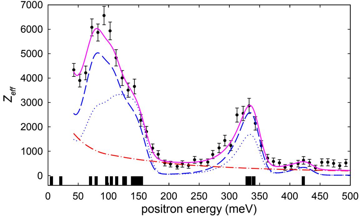
**Figure B.7:** Annihilation spectrum for ethanol ( $\text{CH}_3\text{CH}_2\text{OH}$ ):  $\varepsilon_b = 30 \pm 1$  meV and  $\eta = 0.83$ . Data shown here represent new measurements. Original measurements are shown in Ref. [33].
