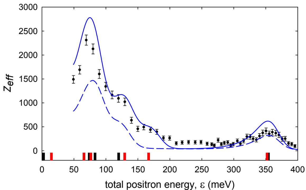
**Figure 4.2:** Annihilation spectrum for 1,2-trans-dichloroethylene ( $C_2H_2Cl_2$ ); ( $\bullet$ ) measured data, ( $--$ ) GL model from Eq. (A.8) with  $\varepsilon_b = 29$  meV using infrared-active modes only and ( $-$ ) GL model using all modes. Vertical bar positions represent vibrational mode energies downshifted by the binding energy, and heights represent mode degeneracies. Black and red indicate infrared-active and inactive modes, respectively.
