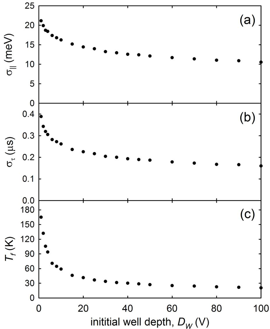
**Figure 5.12:** Effect of well depth on simulated beam. Standard deviation of the (a) parallel energy and (b) temporal distributions obtained from the simulation using a variety of initial well depths,  $D_W \equiv V_E - V_W(0)$ . Also shown in (c) is the final parallel temperature,  $T_f$ . All other parameters as in Fig. 5.8.
