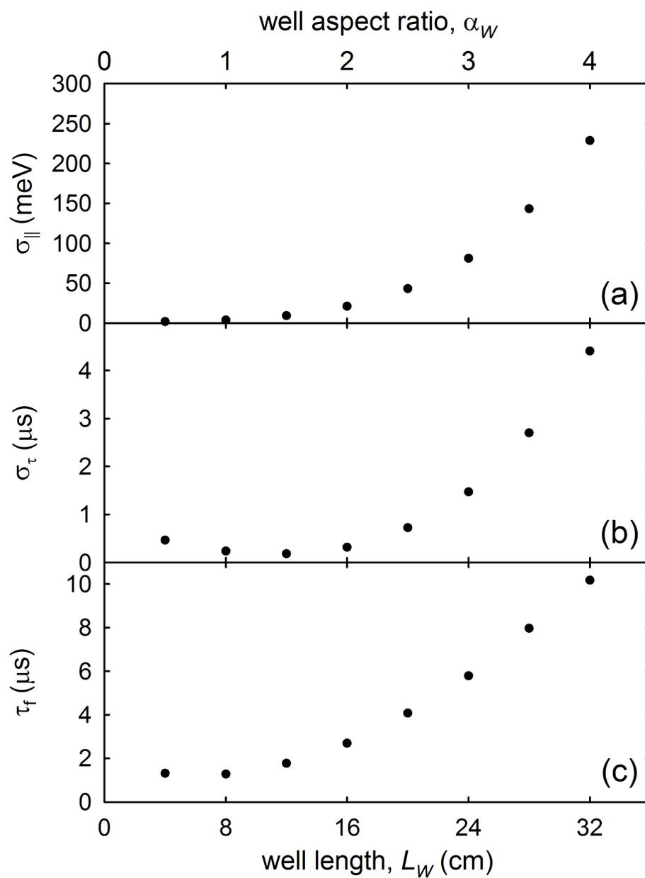
**Figure 5.15:** Effect of well length on simulated beam. Standard deviation of the (a) parallel energy, and (b) time distributions obtained from the simulation of beams produced by traps with a variety of well electrode lengths. Shown in (c) is the average final bounce time during particle ejection. All other parameters as in Fig. 5.8.
