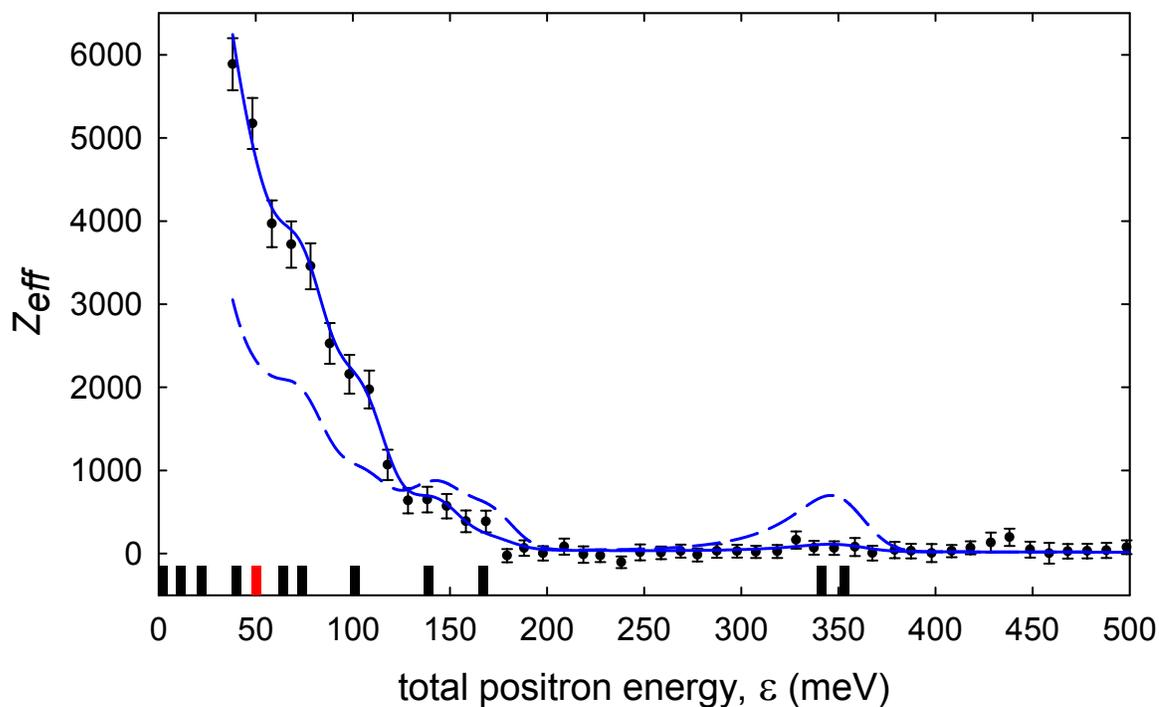
**Figure 4.4:** Annihilation spectrum of 1,1-dichloroethylene (C<sub>2</sub>H<sub>2</sub>Cl<sub>2</sub>); (•) measured data with the fitted MRA component subtracted for clarity, (---) GL model from Eq. (A.8) with  $\epsilon_b = 31$  meV, (—) scaled GL model from Eq. (A.15). Vertical bar positions represent vibrational mode energies downshifted by the binding energy and heights represent mode degeneracies, where black and red indicate infrared-active and inactive modes, respectively.
