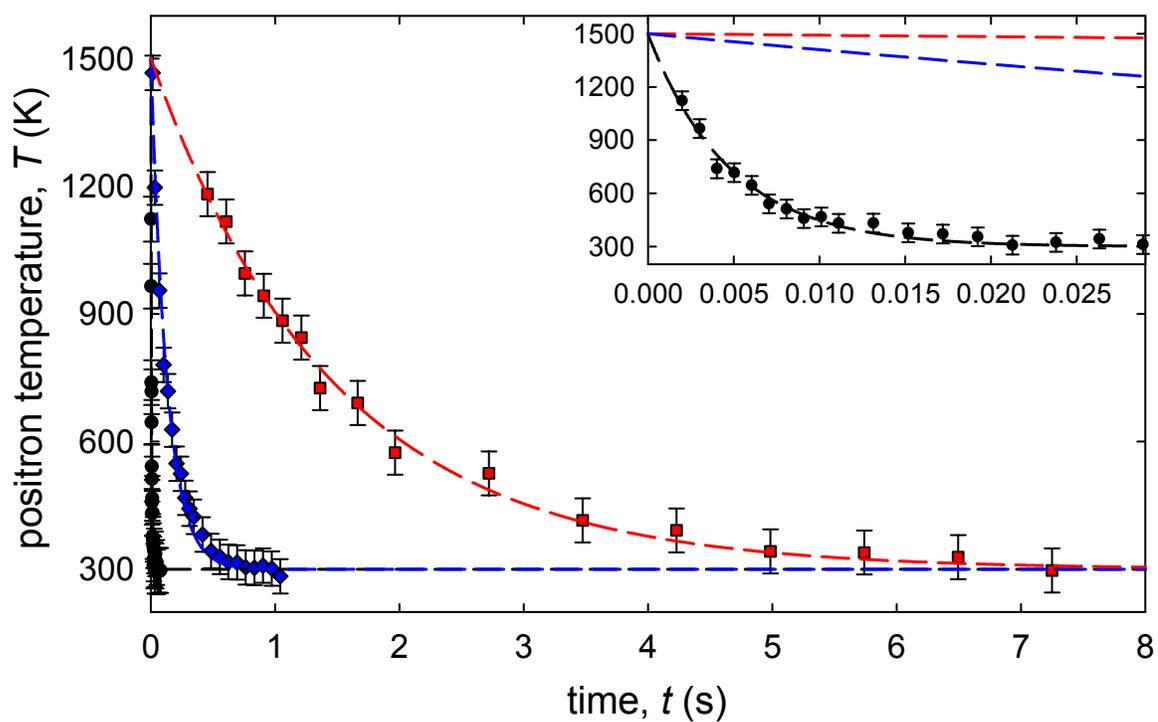
**Figure 6.6:** Positron cooling comparisons at 300 K using (●) CF<sub>4</sub>, (◆) CO, and (■) N<sub>2</sub> gases normalized to 1  $\mu$ torr and shifted to line up at t=0 s; and (---) an exponential fit for each case. The inset shows CF<sub>4</sub> in more detail.
