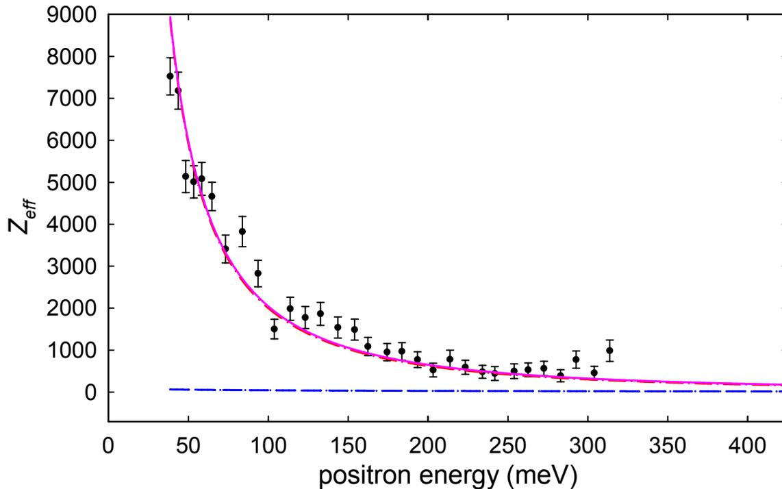
**Figure B.21:** Annihilation spectrum for carbon tetrabromide ( $\text{CBr}_4$ ):  $\epsilon_b = 115$  meV and  $\eta = 0.13$ . Due to lack of resonances, the binding energy is estimated using Eq. 5 of Ref. [83]. Possible energy shifts present.
