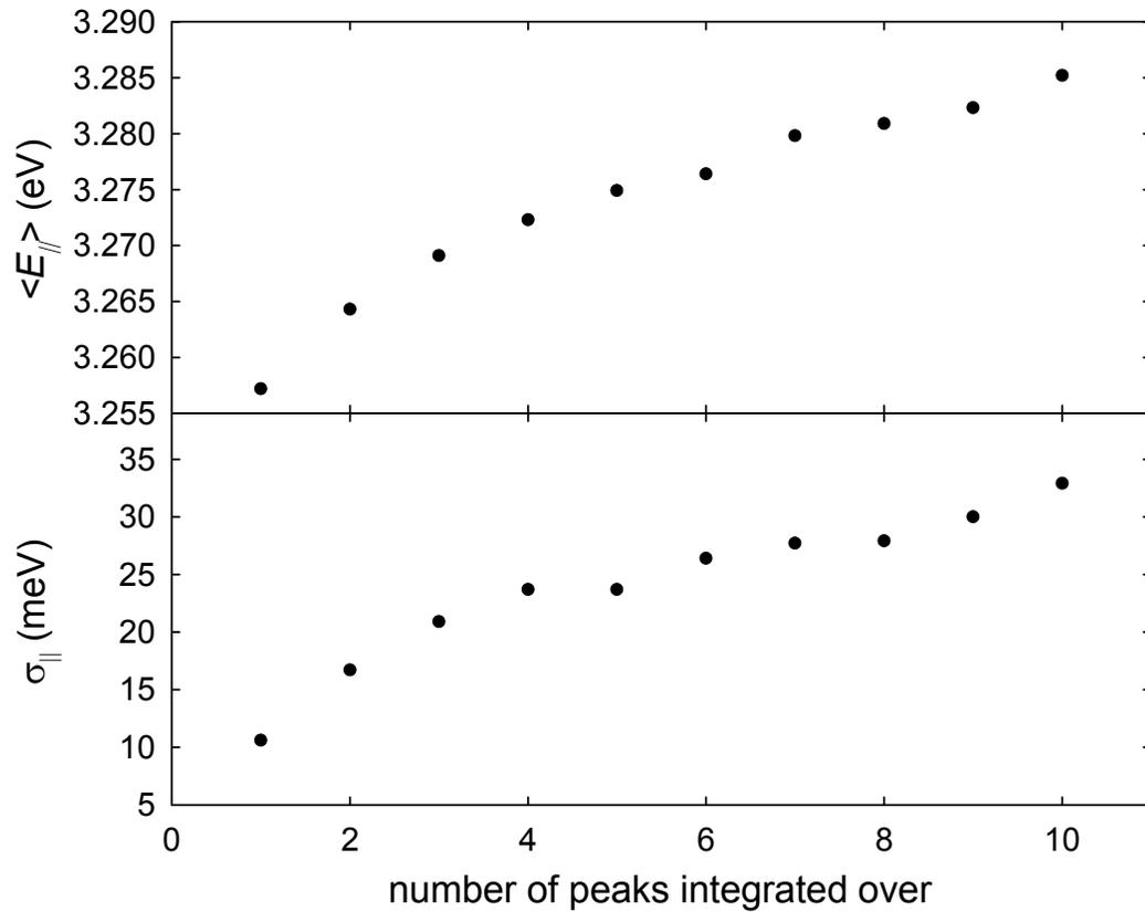
**Figure 3.8:** Effect of beam reflections on measured parallel energy distribution. (a) mean and (b) standard deviation of the parallel energy distribution as the time window of integration is increased to include multiple peaks (i.e., “secondary” beams). See text for details.
