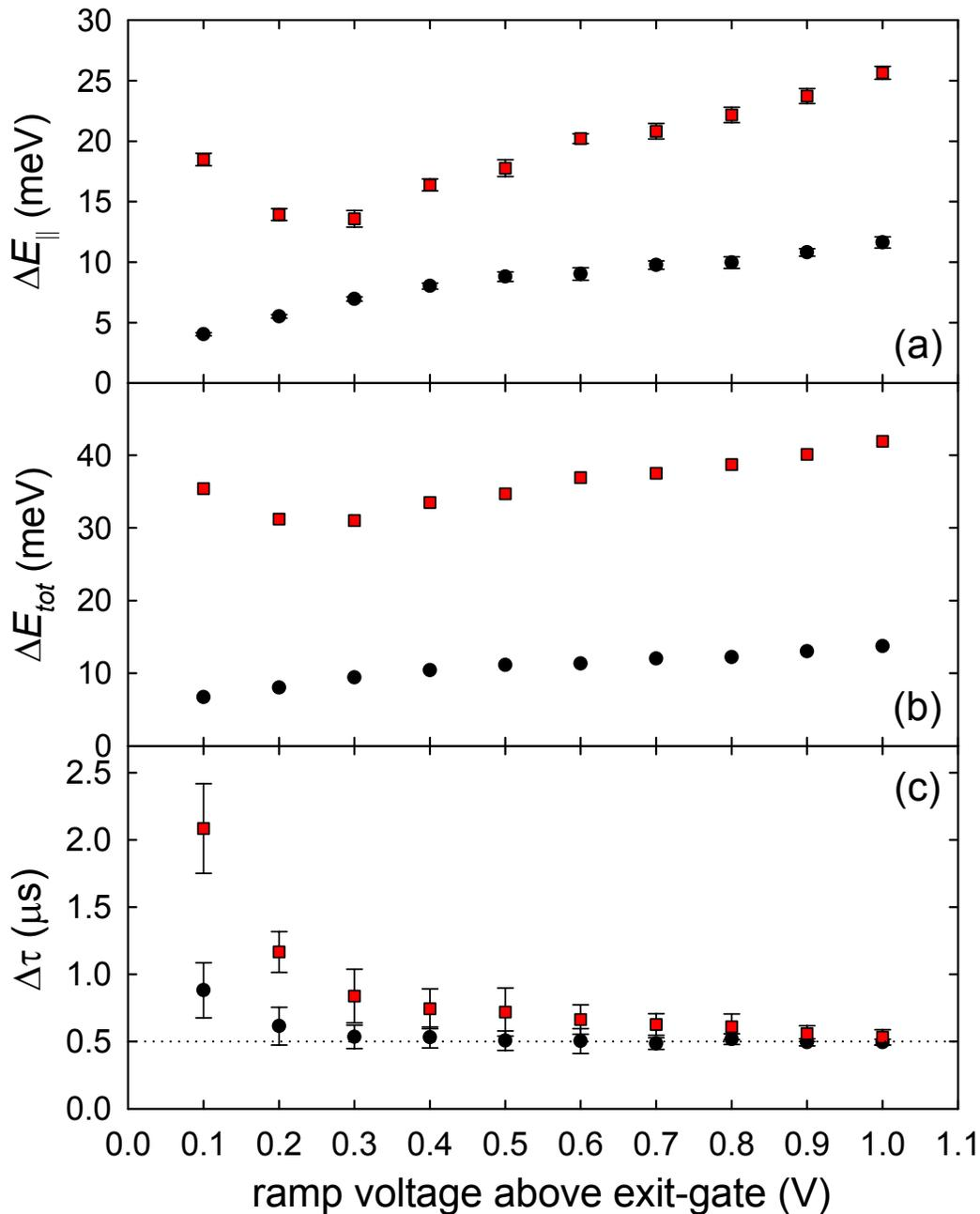
**Figure 7.8:** Effect of ramp voltage on the CBT beam. FWHM of the (a) parallel energy, (b) total energy [calculated using Eq. (3.9)], and (c) time distributions using various ramp voltages,  $\Delta V_r = V_s - V_E$ . ( $\bullet$ ) CBT at  $\sim 300$  K and ( $\blacksquare$ ) CBT at  $\sim 50$  K. Note that in (b) the detector response limits the temporal spread measurement to  $\sim 0.5$   $\mu$ s FWHM (shown by dotted line), and so these values represent upper bounds.
