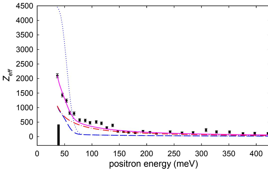
**Figure B.22:** Annihilation spectrum for carbon tetrachloride ( $\text{CCl}_4$ ):  $\varepsilon_b = 57 \pm 1$  meV and  $\eta = 0.09$ . Possible energy shifts present.
