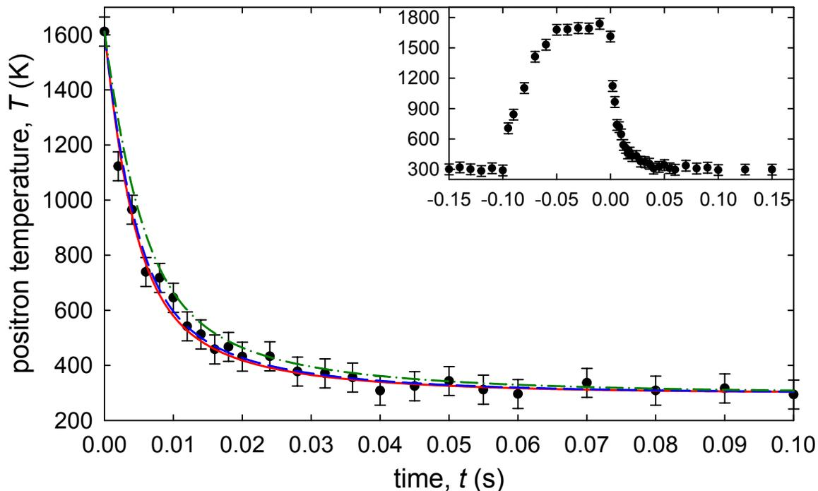
**Figure 6.2:** Positron cooling using  $0.51 \pm 0.05 \mu\text{torr}$  of  $\text{CF}_4$  at 300 K: (●) measured data, (—) solution to Eq. (6.7) for vibrational excitation and de-excitation of the  $\nu_3$  mode, (---) solution to (6.7) with cross sections scaled by a fitting factor  $\eta = 0.95$  and (-·-) solution to Eq. (6.7) with cross sections scaled by  $\eta = 0.75$  to match the direct measurement given in Ref. [41]. Inset shows the full heating and cooling cycle.
