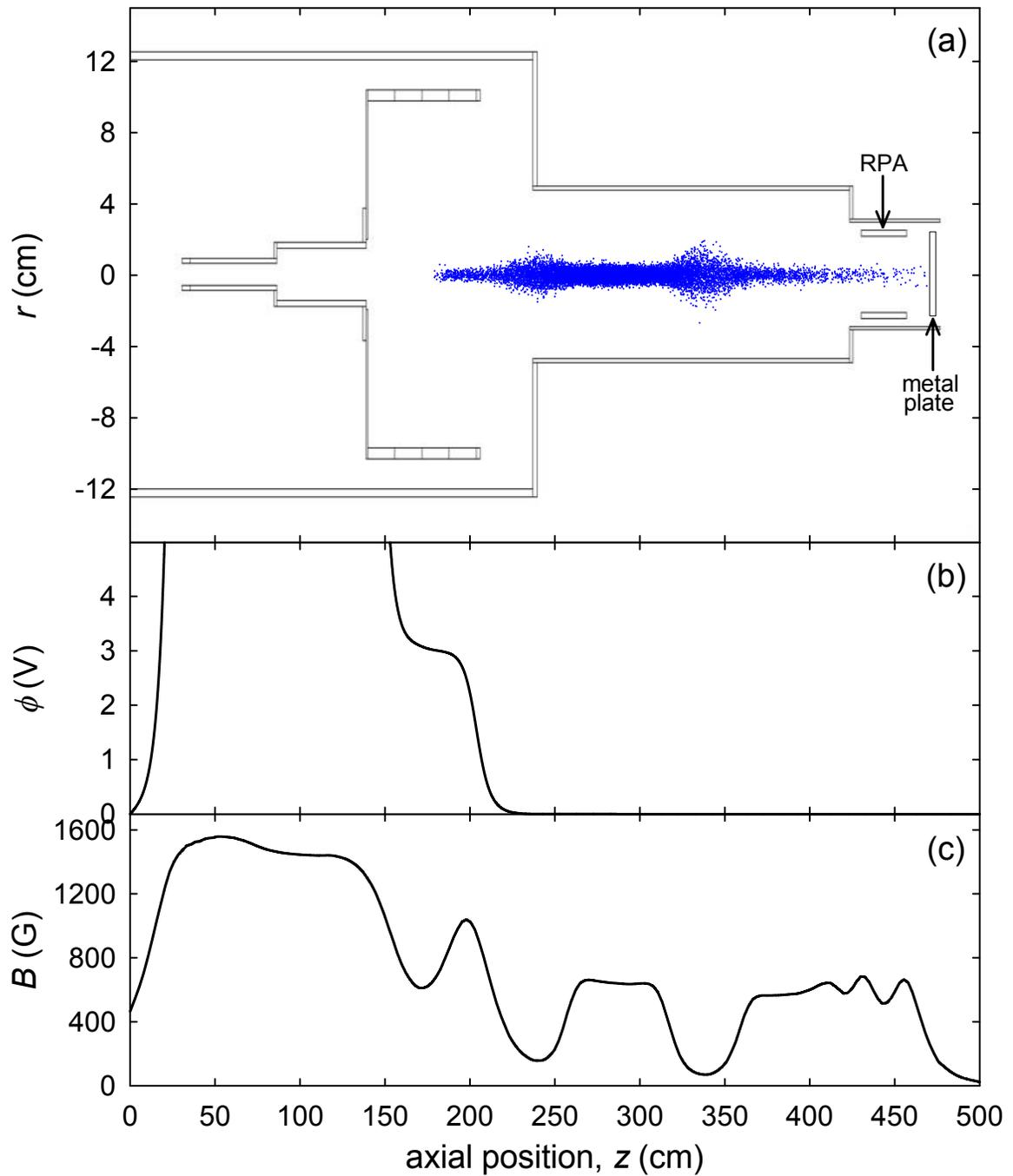
**Figure 5.4:** BGT-based beamline simulation beam transport. (a) electrode geometry with (•) positron axial and radial positions, (b) on-axis potential, and (c) on-axis magnetic field at  $t = 22 \mu\text{s}$ , under the conditions described in Fig. 5.1 and 5.2.
