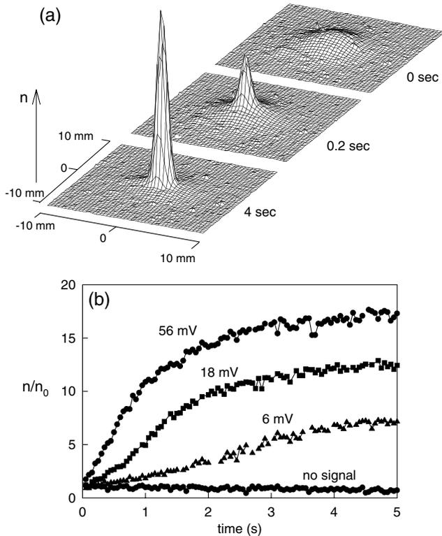
FIG. 2. (a) Radial profiles of a positron plasma with  $N_{\text{tot}} = 10^7$  positrons,  $f_w = 2.5$  MHz,  $A_w = 56$  mV, and  $2 \times 10^{-8}$  torr of  $\text{CF}_4$ . (b) Time evolution of the central density, normalized to its initial value for various values of the applied amplitude.
