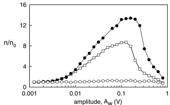
FIG. 4. Compression for cooling on  $\text{CF}_4$  with  $N_{\text{tot}} = 5 \times 10^6$  positrons and  $f_w = 2.5$  MHz for 1 s: ( $\bullet$ )  $P = 4 \times 10^{-8}$  torr; ( $\square$ )  $P = 2 \times 10^{-8}$  torr; ( $\circ$ ) no cooling gas.
