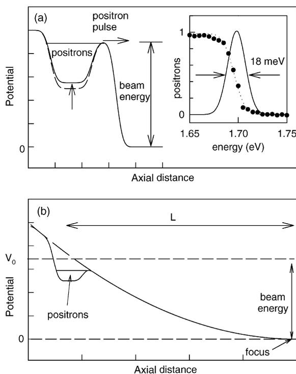
Fig. 2. Electrostatic potential profiles for beam formation using traps: (a) simplest configuration with asymmetrical well and fixed potential exit gate potential. The inset shows a typical parallel energy distribution obtainable using room temperature positrons; (b) the harmonic potential geometry, as described in text.
