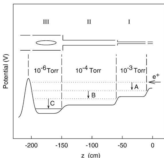
Fig. 1. Schematic diagram of a gas-buffered positron trap, showing the three stages of differential pumping and the electrostatic potential.
