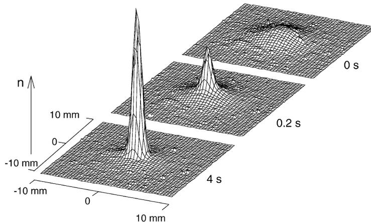
Fig. 3. Radial profiles of a positron plasma following the application of a rotating electric field at  $t = 0$ . Conditions were:  $N_{\text{tot}} = 10^7$  positrons, signal frequency,  $f_w = 2.5$  MHz, signal amplitude  $A_w = 56$  mV. The cooling gas was  $\text{CF}_4$  at a pressure of  $2 \times 10^{-8}$  Torr.
