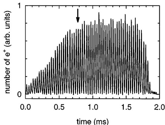
FIG. 2. A pulse train of 60 pulses, each consisting of approximately  $10^5$  positrons, shows the ramp-up, flat-top, and terminal phases of the pulse envelope, which is independent of the specific number of pulses. The energy distribution shown in Fig. 3 was obtained for a pulse at the beginning of the flat-top portion of an equivalent envelope (see arrow).
