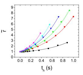
FIG. 12. Plasma radius, normalized to the radius for  $t_h = 0$ , as a function of hold time  $t_h$  at various displacements by varying  $t_a$  at constant chirp rate, k = 2.5 kHz/s: (**I**)  $d/r_w = 0.43$ , (**O**)  $d/r_w = 0.52$ , (**A**)  $d/r_w = 0.63$ , (**V**)  $d/r_w = 0.67$ , (**A**)  $d/r_w = 0.70$ , and (**b**)  $d/r_w = 0.76$ . The data at each displacement (–) are fit with separate exponential functions to extract the expansion rate,  $\Gamma(d)$ .
