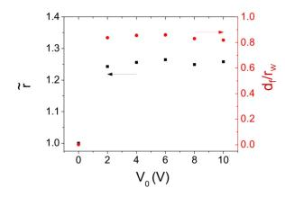
FIG. 10. (**■**) Variation of plasma radius (normalized to the initial radius) with drive amplitude  $V_0$ , applied for a fixed time  $t_a$  at constant chirp rate k; and (**●**) the corresponding displacement  $d_d r_w$ .
