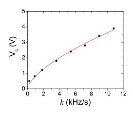
FIG. 5. Critical drive voltage to excite a typical long plasma to  $0.65 \le d/R_w < 0.8$  for various chirp rates k. The fit (–) corresponds to  $V_c \propto k^{0.65\pm0.03}$ .
