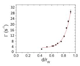
FIG. 13. Plasma expansion rate, calculated from the fits in Fig. 12, as a function of  $d/r_w$ . Also shown (–) is the fit to the data. See text for details.
