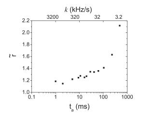
FIG. 11. Final plasma radius, at  $d_f/r_w = 0.82$ , normalized to the initial radius at d=0, as a function of the autoresonant time  $t_a$ , on a semilogarithmic scale, for a plasma with  $L_p \sim 4$  cm.
