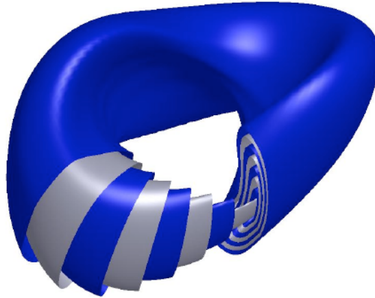
Fig. 5.21. The magnetic field topology in the CNT stellarator. Field lines on each of the (colored) surfaces remain on that surface as they transit both the long way and short way around the device. It is this twist of the field lines, which are induced by the external field coils shown in Figure 5.21, that stabilizes the confined plasma. Drawing courtesy of T. S. Pedersen.
